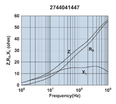
Impedance, reactance, and resistance vs. frequency.
