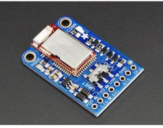
Bluefruit LE UART Friend or Flora BLE If you have a stand-alone UART module you have some flexibility with wiring. However we suggest **hardware UART** if possible. You will likely need to use the flow control **CTS** pin if you are not using hardware UART. There's also a **MODE** pin
