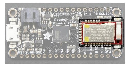
Since not all pins can be brought out to breakouts, due to the small size of the Feather, we use these to control the BLE module
