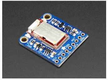
Bluefruit LE SPI Friend If you have a stand-alone module, you have a bit of flexibility with wiring however we strongly recommend Hardware SPI, CS = 8, IRQ = 7, RST = 4
