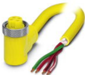
Sensor/actuator cable, 4-position, PVC, yellow, free cable end, on Socket angled 7/8"-16UNF, A-coded, cable length: 6 m
