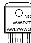
D 2 PAK 5 CASE 936A ADJUSTABLE
