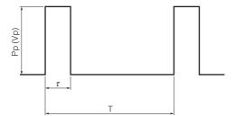
$P_P$  : Pulse limit power (W)  $V_P$  : Pulse limit voltage (V)  $\tau$  : Pulse continuous time (s)
