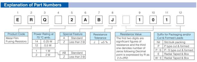
The above example shows a standard Metal Film Fusing Resistors, 2 W power rating, resistance value of 100  $\Omega$ , tolerance of  $\pm 5$  %, and package of standard bulk packing.
