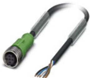
Sensor/actuator cable, 5-position, PUR, black-gray RAL 7021, free cable end, on Socket straight M12, A-coded, cable length: 10 m
