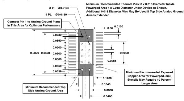
Figure 10. Recommended Land Pattern for 28-Pin PWP PowerPAD
