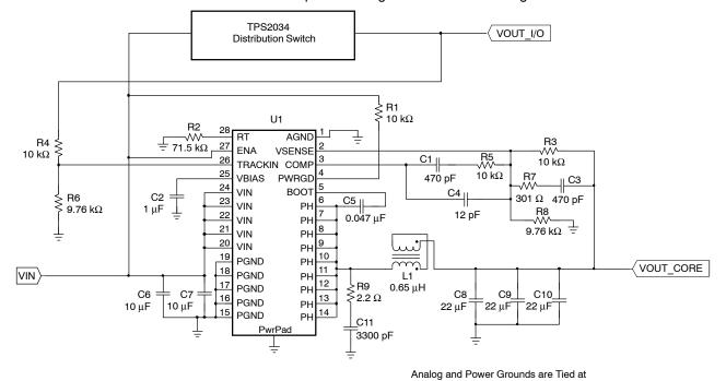
Figure 20. Typical Application With Power Switch
