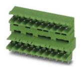
Header, Nominal current: 10 A, Rated voltage (III/2): 320 V, Number of positions: 2, Pitch: 5.08 mm, Color: green, Contact surface: Tin, Mounting: Wave soldering, The article can be aligned to create different nos. of positions! In combination with MVSTB or FKCV plug components, both an MVSTBW (or FKCVW) and an MVSTBR plug (or FKCVR) must be used. Combination with TMSTBP plug components is not possible!
