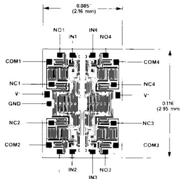
NOTE: NC<sub>x</sub> IS CONNECTED TO COM<sub>x</sub> WHEN IN<sub>x</sub> IS LOW.
