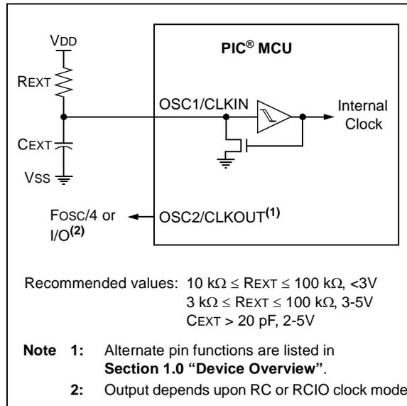
In RCIO mode, the RC circuit is connected to OSC1. OSC2 becomes an additional general purpose I/O pin. The RC oscillator frequency is a function of the supply voltage, the resistor ( $R_{EXT}$ ) and capacitor ( $C_{EXT}$ ) values and the operating temperature. Other factors affecting the oscillator frequency are:
