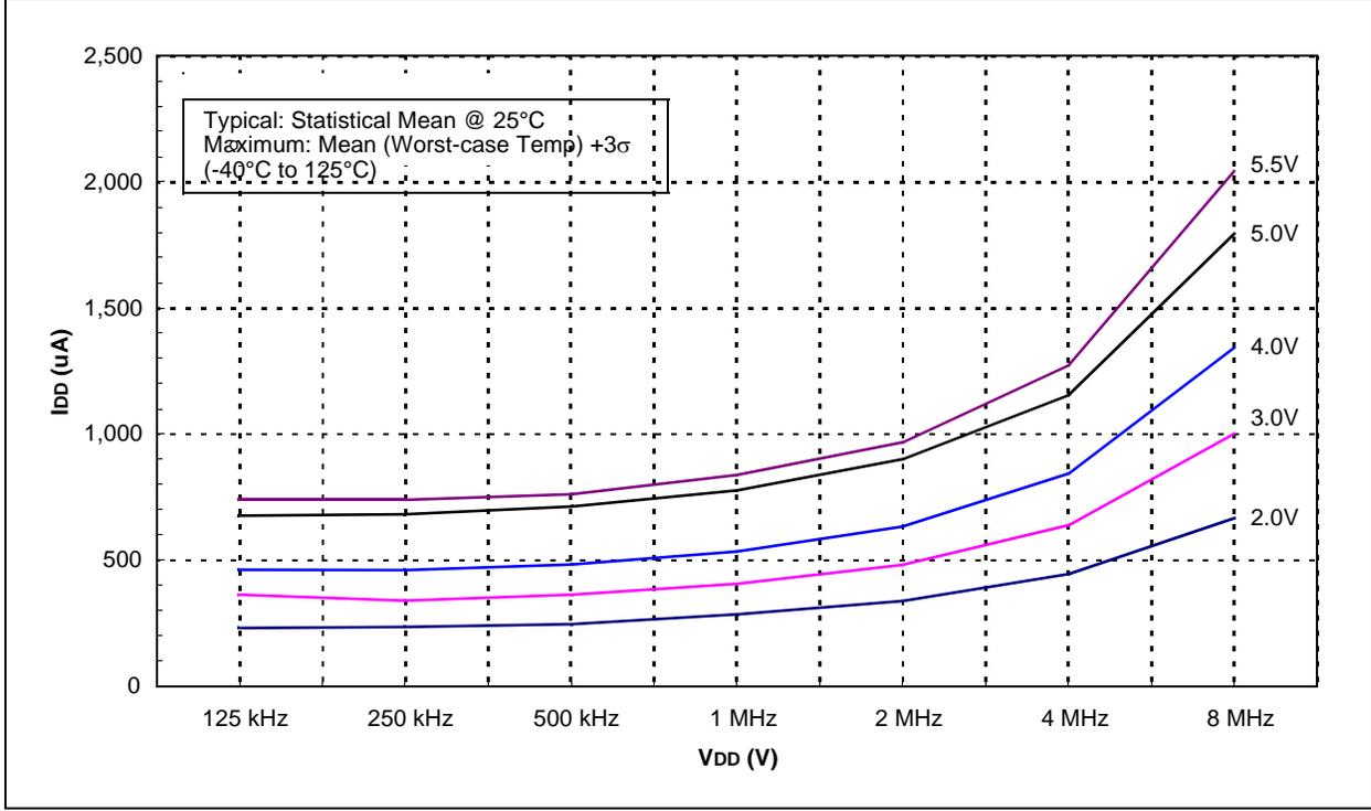
FIGURE 15-13: TYPICAL I<sub>PD</sub> vs. V<sub>DD</sub> (SLEEP MODE, ALL PERIPHERALS DISABLED)
