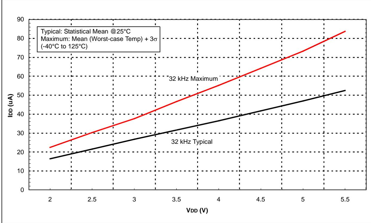
FIGURE 15-11: TYPICAL  $I_{DD}$  vs.  $F_{OSC}$  OVER  $V_{DD}$  (HFINTOSC MODE)
