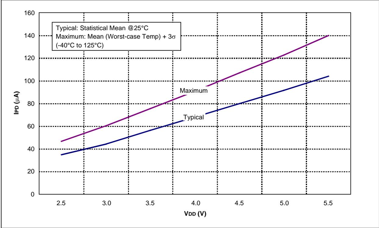
FIGURE 15-17: TYPICAL WDT IPD vs. VDD (25°C)
