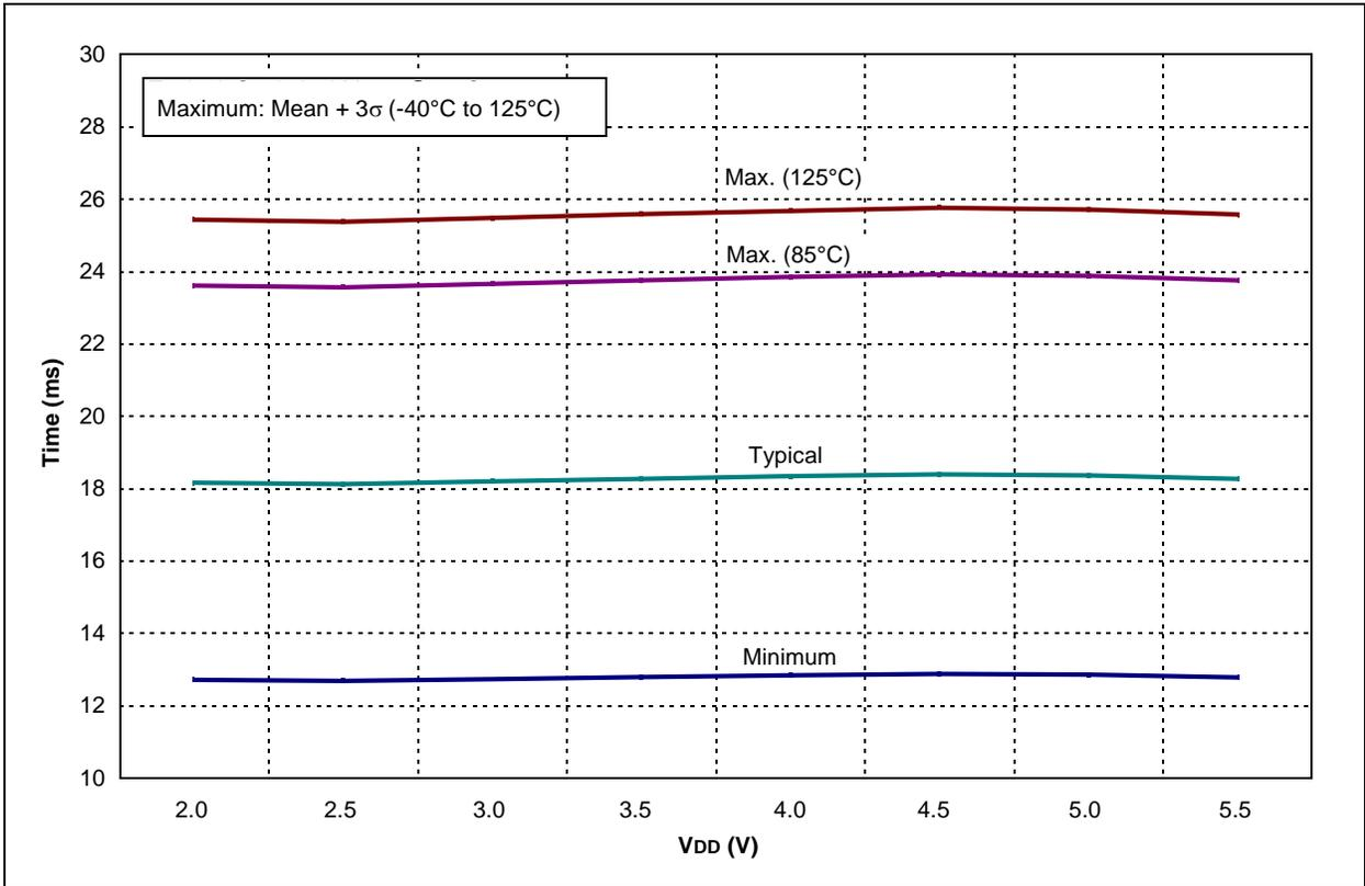
FIGURE 15-20: WDT PERIOD vs. TEMPERATURE
