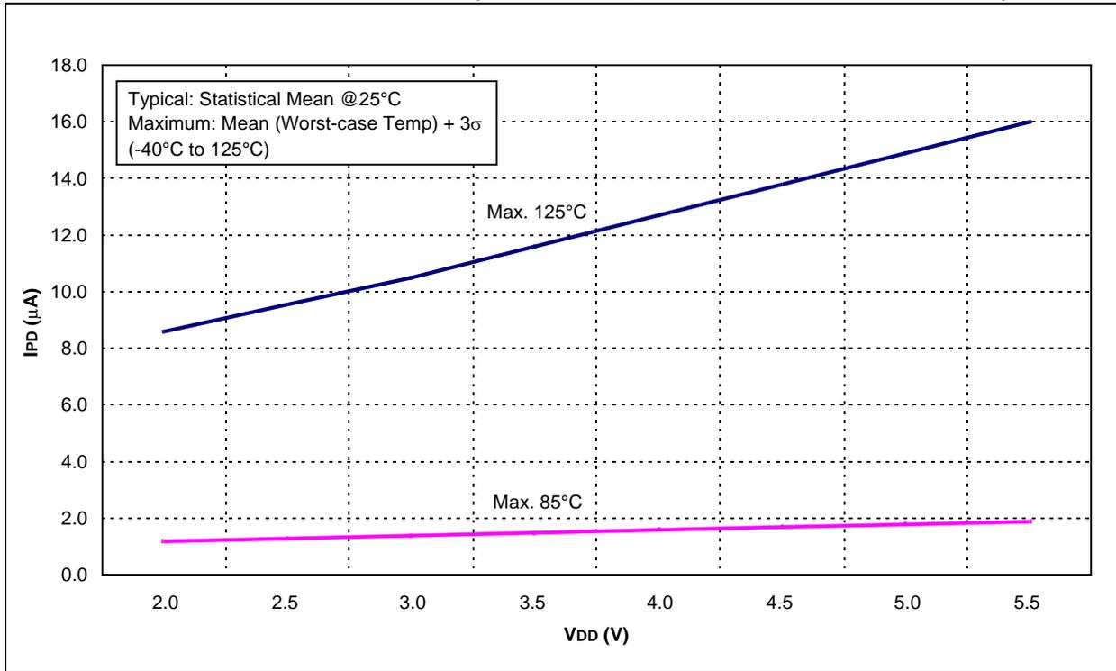
**FIGURE 15-15: COMPARATOR IPD vs. VDD (BOTH COMPARATORS ENABLED)**
