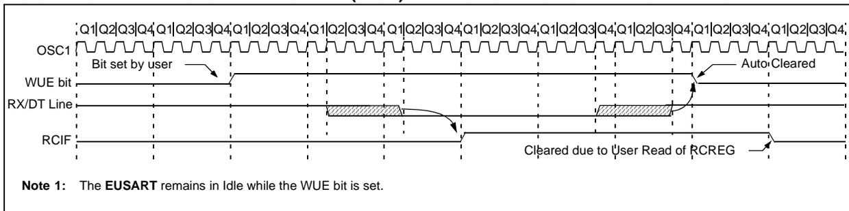
**FIGURE 10-8: AUTO-WAKE-UP BIT (WUE) TIMINGS DURING SLEEP**
