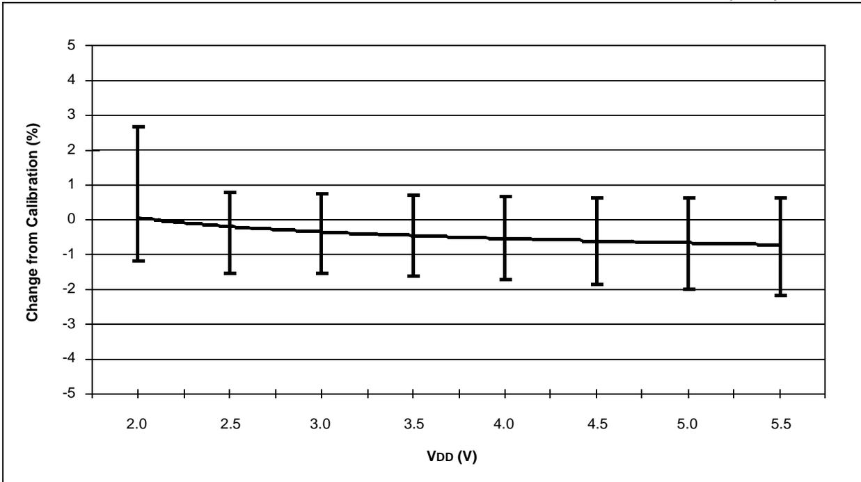
**FIGURE 15-39: TYPICAL HFINTOSC FREQUENCY CHANGE vs. V<sub>DD</sub> (125°C)**
