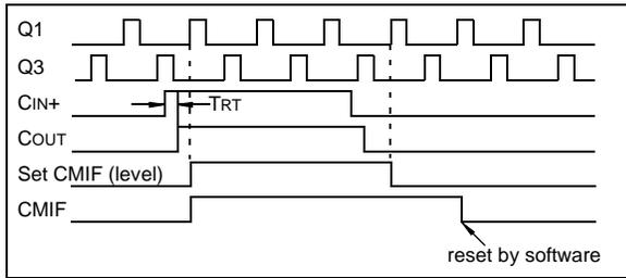
**FIGURE 7-7: COMPARATOR INTERRUPT TIMING WITH CMCON0 READ**
