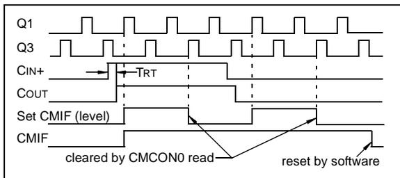
**Note 1:** If a change in the CM1CON0 register (CxOUT) occurs when a read operation is being executed (start of the Q2 cycle), then the CxIF Interrupt Flag bit of the PIR1 register may not get set.
