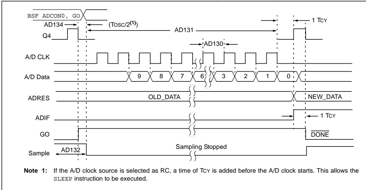
**FIGURE 14-10: PIC16F688 A/D CONVERSION TIMING (SLEEP MODE)**
