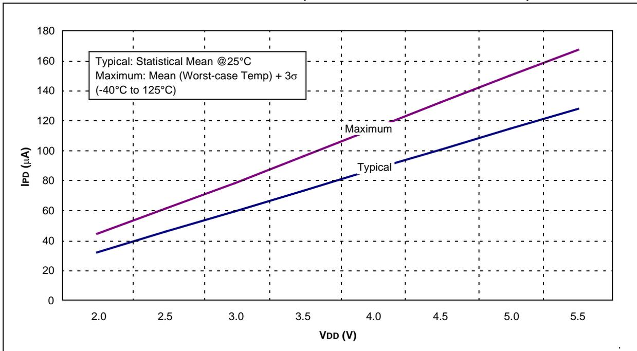
FIGURE 15-16: BOR IPD vs. VDD OVER TEMPERATURE
