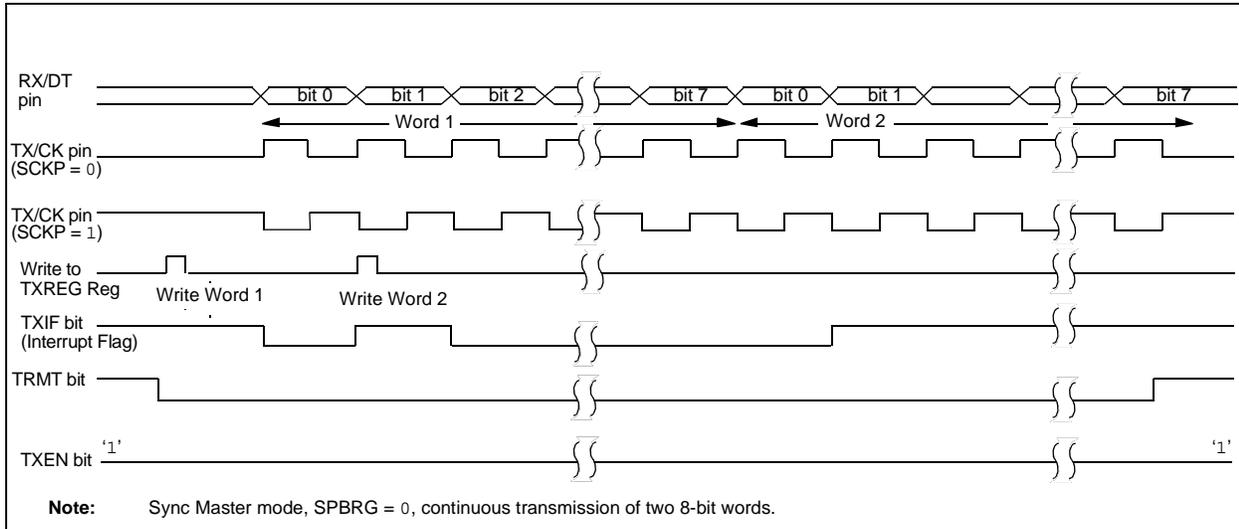
**FIGURE 10-11: SYNCHRONOUS TRANSMISSION (THROUGH TXEN)**
