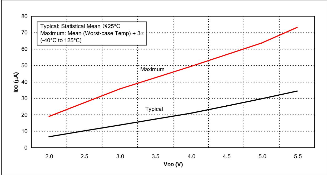
FIGURE 15-10:  $I_{DD}$  vs.  $V_{DD}$  (LP MODE)
