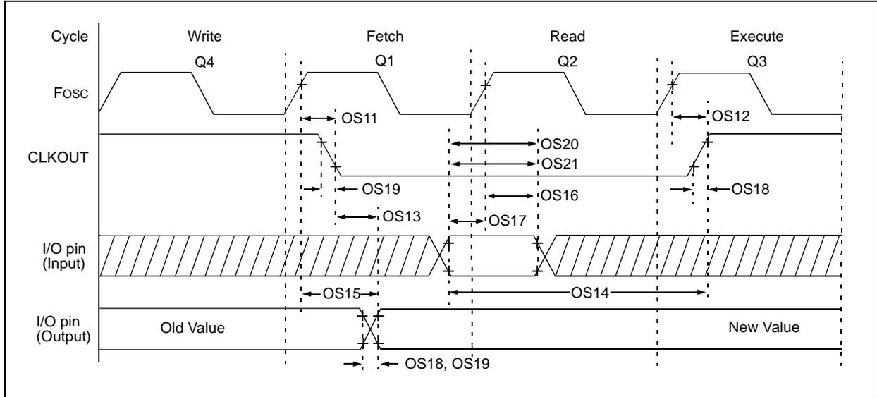
**TABLE 14-3: CLKOUT AND I/O TIMING PARAMETERS**
