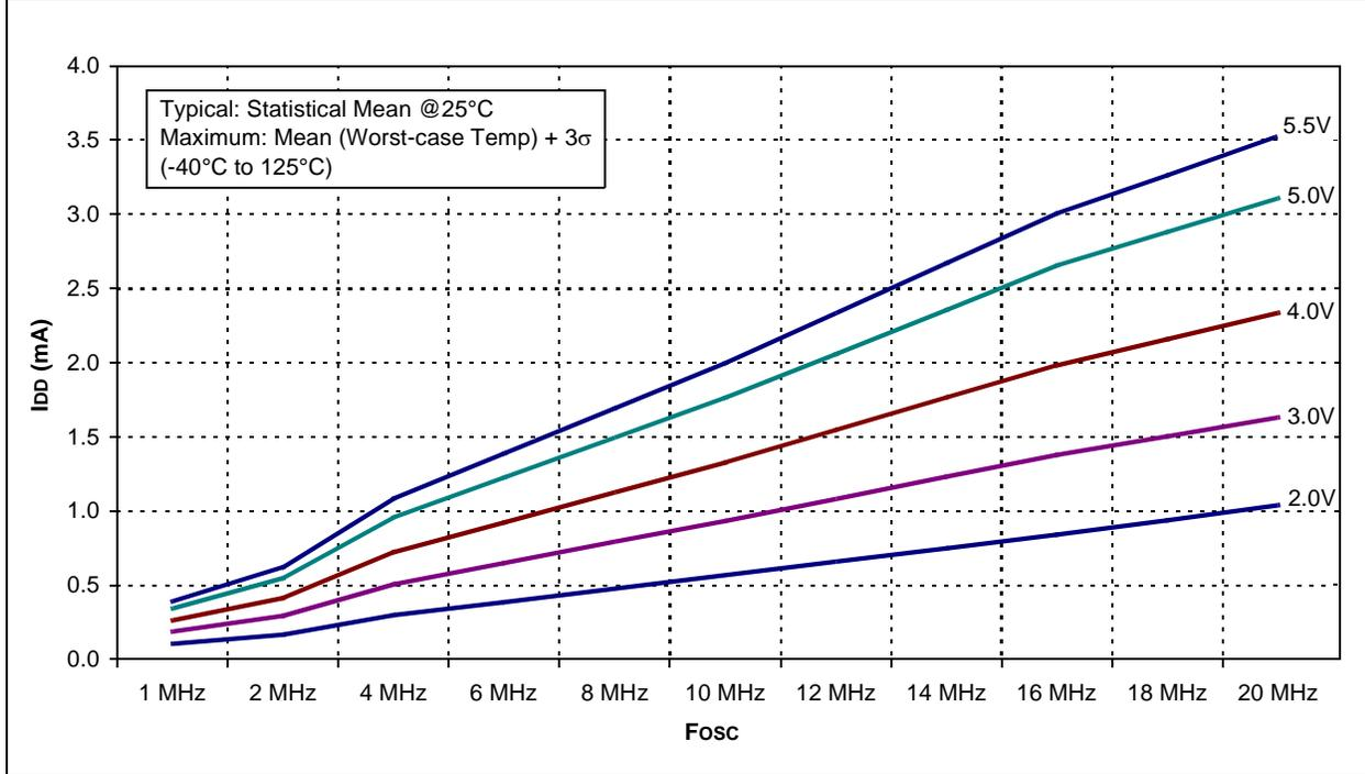
FIGURE 15-3: TYPICAL I<sub>DD</sub> vs. F<sub>osc</sub> OVER V<sub>DD</sub> (HS MODE)
