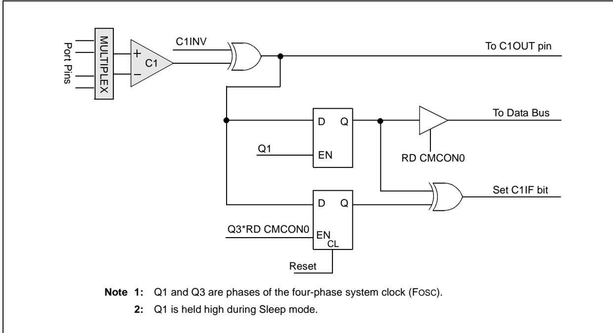
**FIGURE 7-3: COMPARATOR C2 OUTPUT BLOCK DIAGRAM**
