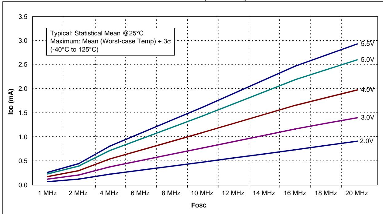
FIGURE 15-2: MAXIMUM I<sub>DD</sub> vs. F<sub>osc</sub> OVER V<sub>DD</sub> (EC MODE)
