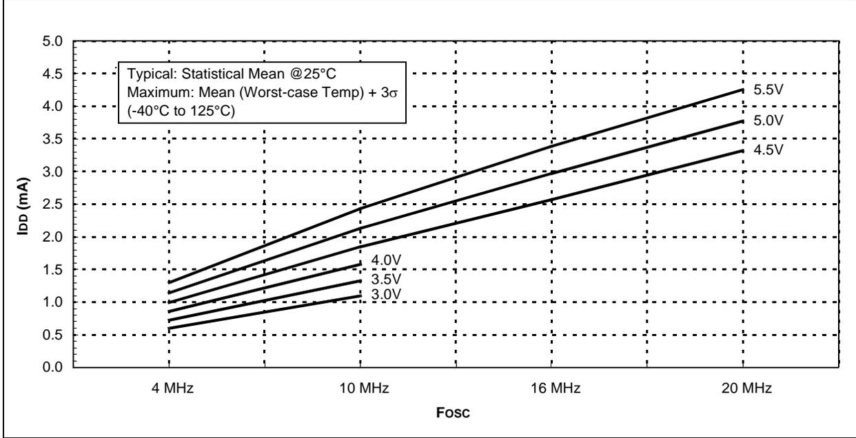
FIGURE 15-5: TYPICAL I<sub>DD</sub> vs. V<sub>DD</sub> OVER F<sub>osc</sub> (XT MODE)
