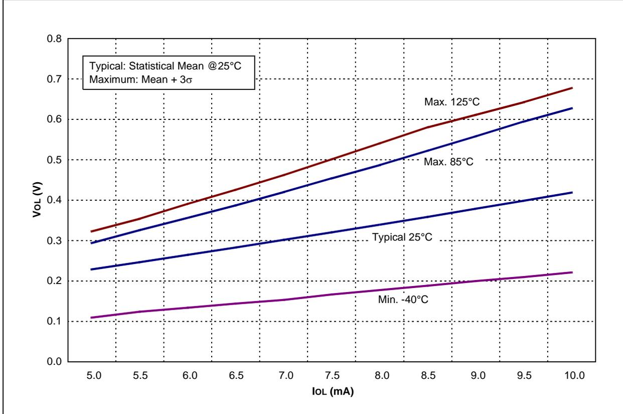
**FIGURE 15-24:  $V_{OL}$  vs.  $I_{OL}$  OVER TEMPERATURE ( $V_{DD} = 5.0V$ )**
