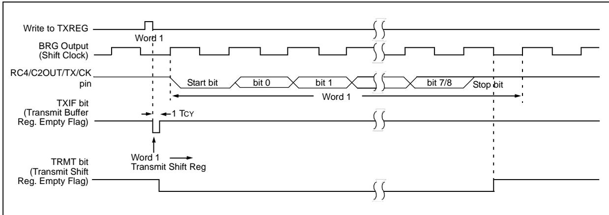
**FIGURE 10-4: ASYNCHRONOUS TRANSMISSION (BACK-TO-BACK)**
