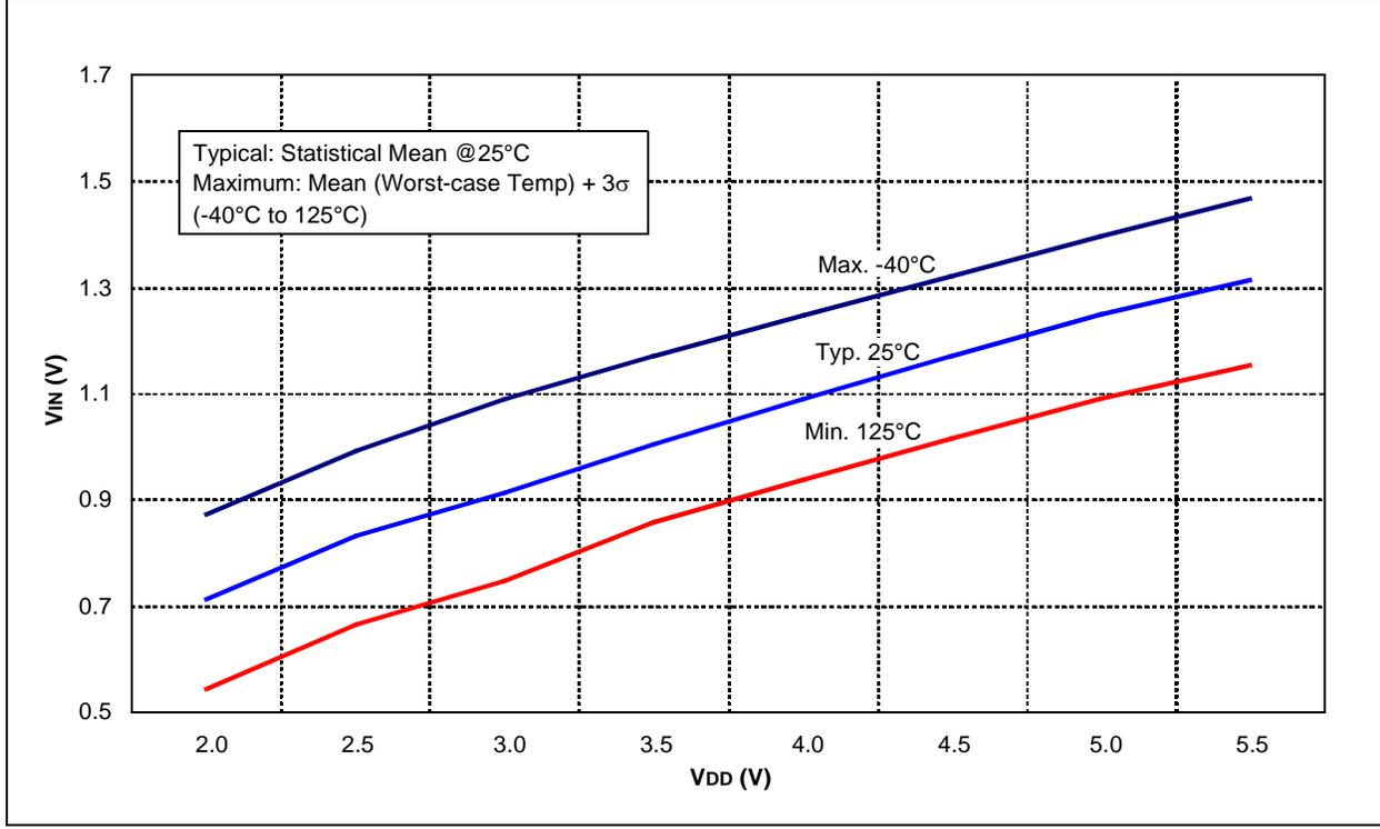
FIGURE 15-28: SCHMITT TRIGGER INPUT THRESHOLD  $V_{IN}$  vs.  $V_{DD}$  OVER TEMPERATURE
