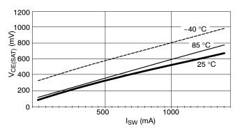
Figure 5.  $V_{CE(SAT)}$  vs.  $I_{SW}$
