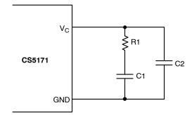
Figure 31. A Typical Compensation Network
