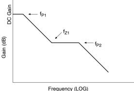
Figure 32. Bode Plot of the Compensation Network Shown in Figure 31
