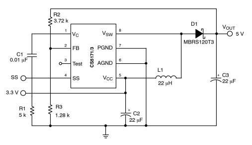
Figure 1. Applications Diagram
