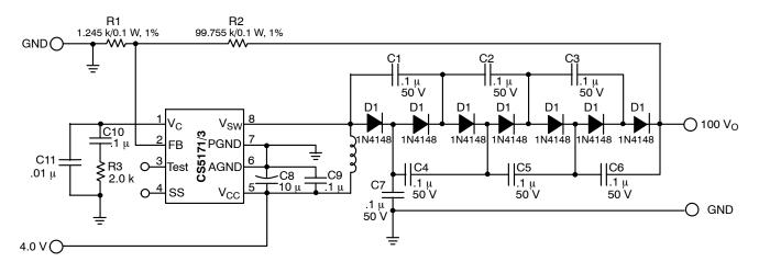
Figure 46. Additional Application Diagram, 4.0 V Input, 100 V/ 10 mA Output Boost Converter with Output Voltage Multiplier
