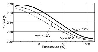
Figure 15. Current Limit vs. Temperature
