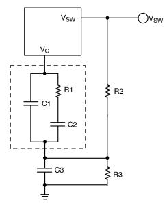
Figure 39. Technique for Increasing Slope Compensation
