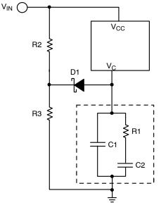
Figure 37. Current Limiting using a Diode Clamp
