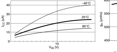
Figure 21. I<sub>CC</sub> vs. V<sub>IN</sub> During Shutdown
