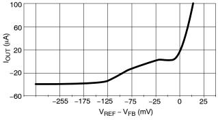
Figure 24. Error Amplifier I<sub>OUT</sub> vs. V<sub>FB</sub> (CS5171/3 only)
