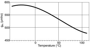
Figure 22. Error Amplifier Transconductance vs. Temperature (CS5171/3 only)
