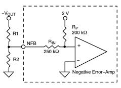
Figure 33. Negative Error Amplifier and NFB Pin
