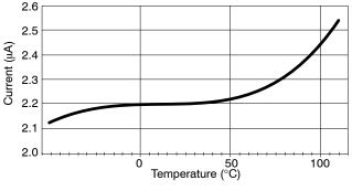
Figure 26. Switch Leakage vs. Temperature
