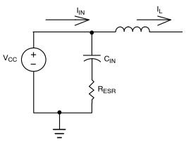
Figure 35. Boost Circuit Effective Input Filter
