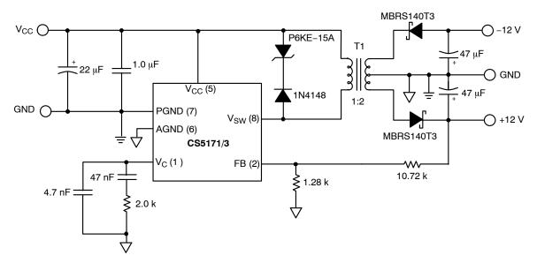
Figure 43. Additional Application Diagram, 2.7 to 13 V Input, ±12 V/ 200 mA Output Flyback Converter
