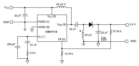
Figure 45. Additional Application Diagram, 2.7 V to 28 V Input, 5.0 V Output SEPIC Converter
