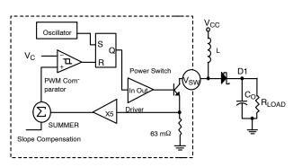
Figure 27. Current Mode Control Scheme
