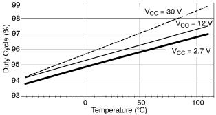
Figure 16. Maximum Duty Cycle vs. Temperature
