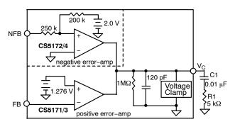
Figure 29. Error Amplifier Equivalent Circuit
