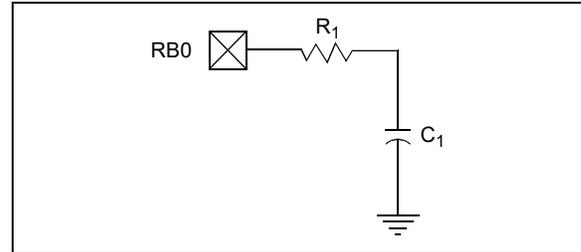
A timer can be used to measure the charge time and discharge time of the capacitor. The charge time can then be adjusted to provide the desired delay in Sleep. This technique compensates for the affects of temperature, voltage and component accuracy. The peripheral can also be configured as a simple, programmable Low-Voltage Detect (LVD) or temperature sensor.
