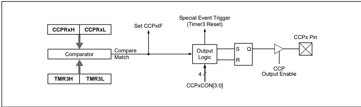
**FIGURE 16-3: SIMPLIFIED PWM BLOCK DIAGRAM**
