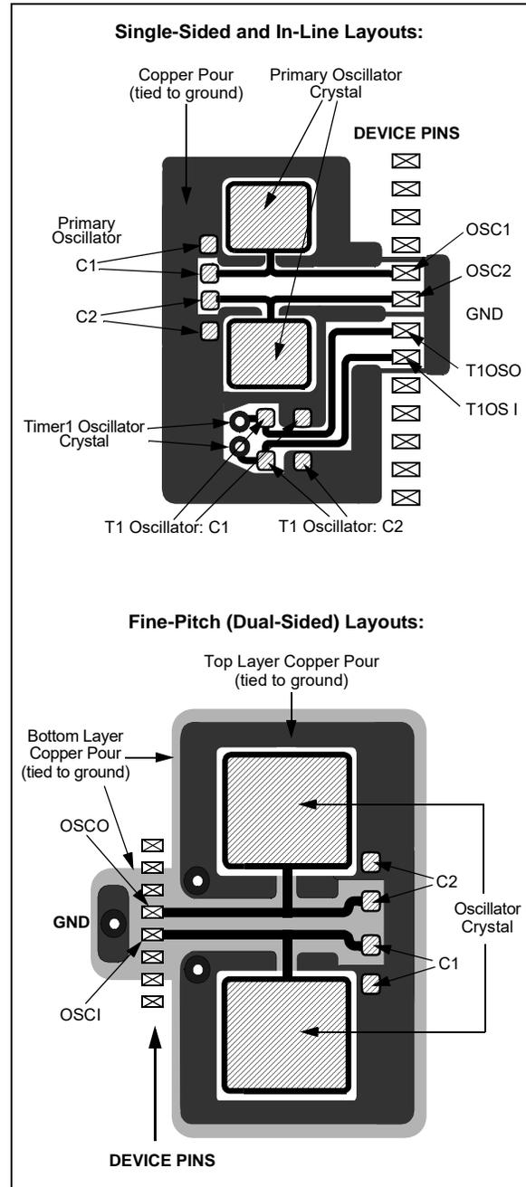
In planning the application's routing and I/O assignments, ensure that adjacent port pins and other signals, in close proximity to the oscillator, are benign (i.e., free of high frequencies, short rise and fall times, and other similar noise).
