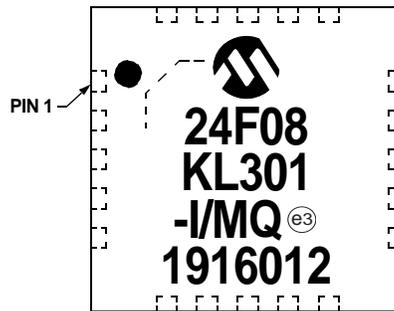
28-Lead QFN (5x5x0.9 mm)
