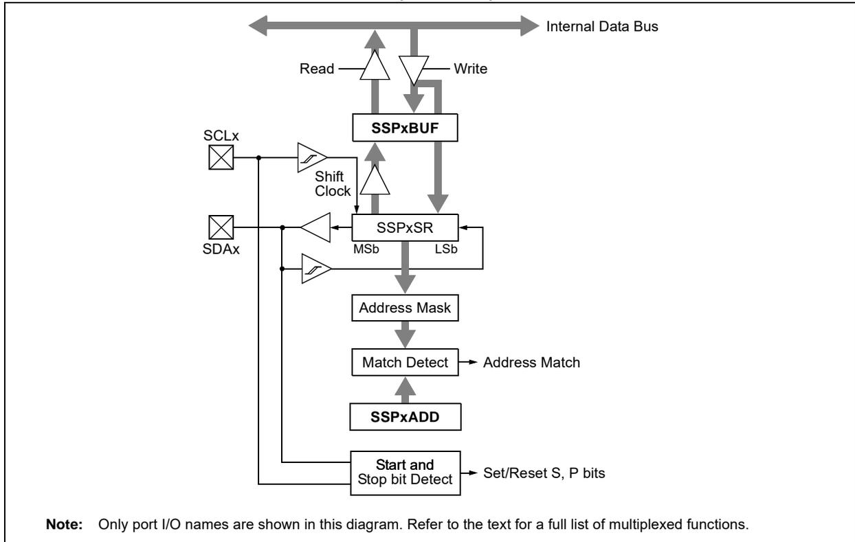
**FIGURE 17-4: MSSPx BLOCK DIAGRAM (I<sup>2</sup>C MASTER MODE)**
