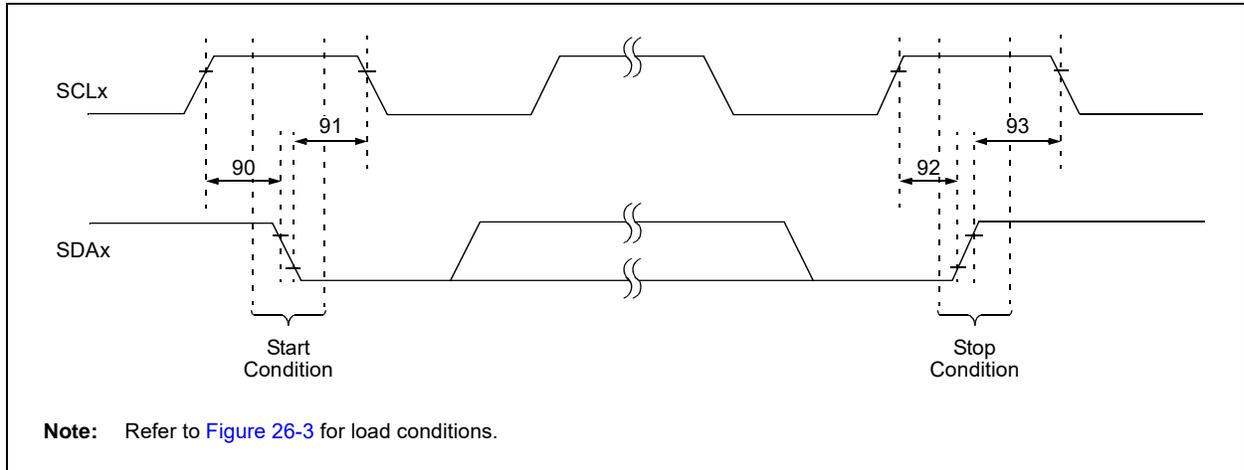
**TABLE 26-33: I<sup>2</sup>C BUS START/STOP BITS REQUIREMENTS (MASTER MODE)**
