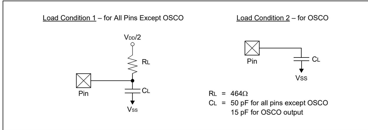
**TABLE 26-17: CAPACITIVE LOADING REQUIREMENTS ON OUTPUT PINS**
