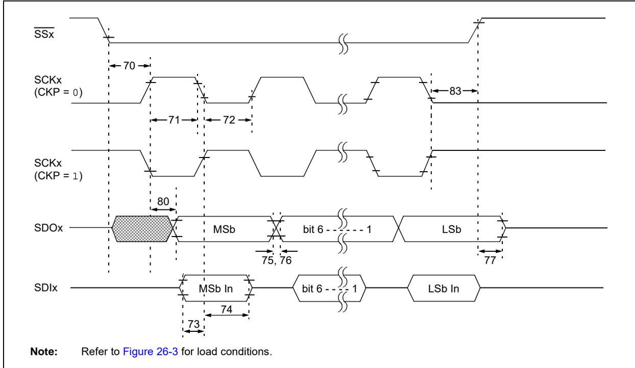
**TABLE 26-29: EXAMPLE SPI MODE REQUIREMENTS (SLAVE MODE TIMING, CKE = 0)**
