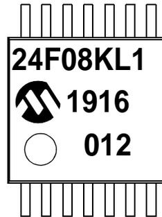
20-Lead SSOP (5.30 mm)
