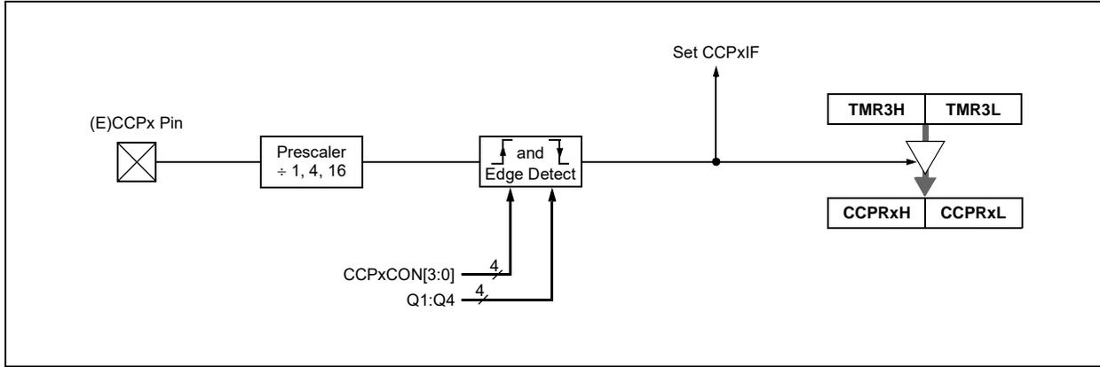
**FIGURE 16-2: GENERIC COMPARE MODE BLOCK DIAGRAM**
