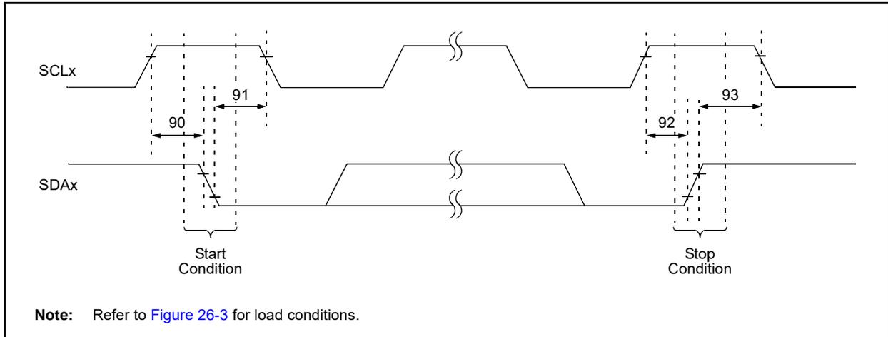
**TABLE 26-31: I<sup>2</sup>C BUS START/STOP BITS REQUIREMENTS (SLAVE MODE)**
