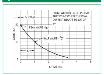
**Figure 3 - Pulse Derating Curve**
