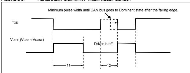
FIGURE 2-10: TIMING DIAGRAM FOR LOOP DELAY SYMMETRY
