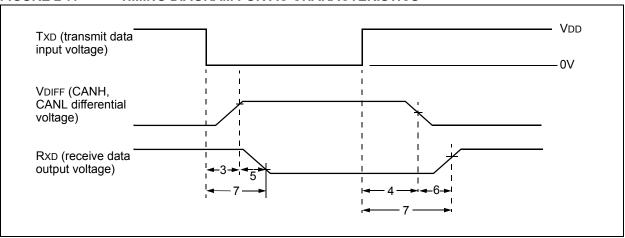
FIGURE 2-8: TIMING DIAGRAM FOR WAKEUP FROM STANDBY
