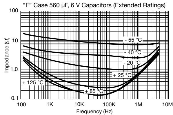
**TYPICAL CURVES OF IMPEDANCE, AS A FUNCTION OF FREQUENCY**
