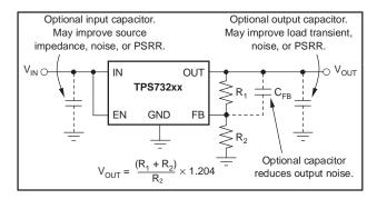
Figure 33. Typical Application Circuit for Adjustable-Voltage Versions
