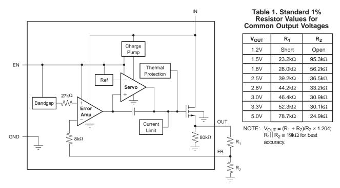
Figure 3. Adjustable Voltage Version
