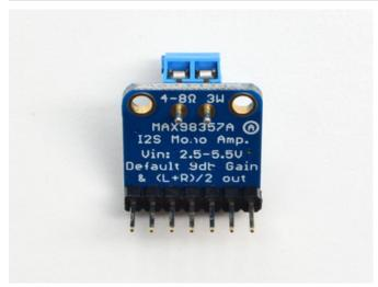
If you want to use a terminal block for connecting a speaker, place the 3.5mm terminal so the mouthes point out.
