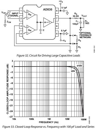
**Resistor Compensation** SUPPLIES, BYPASSING, AND GROUNDING
