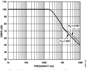
Figure 2. Common-Mode Rejection Ratio vs. Frequency
