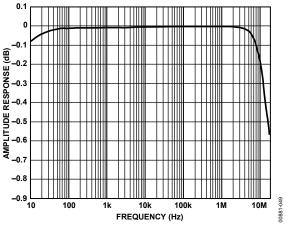
Figure 49. Amplitude Response vs. Frequency for Line Receiver
