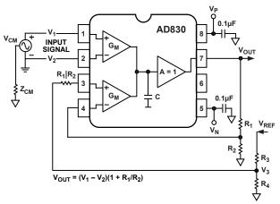
Figure 41. Offsetting the Output with Differential Gain >1
