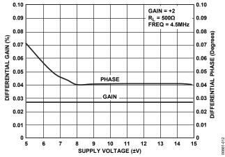
Figure 12. Differential Gain and Phase vs. Supply Voltage,  $R_L = 500 \Omega$
