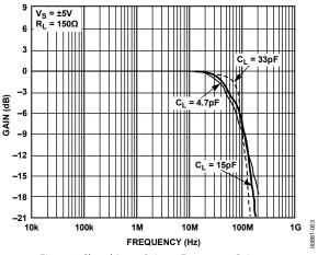
Figure 3. Closed-Loop Gain vs. Frequency, Gain = +1
