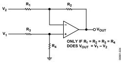
Figure 24. Op Amp Based Difference Amplifier
