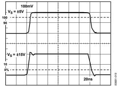
Figure 19. Small Signal Pulse Response,  $R_L = 150 \Omega$ ,  $C_L = 4.7 pF$ , G = +1
