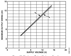
Figure 31. Maximum Output Swing vs. Supply
