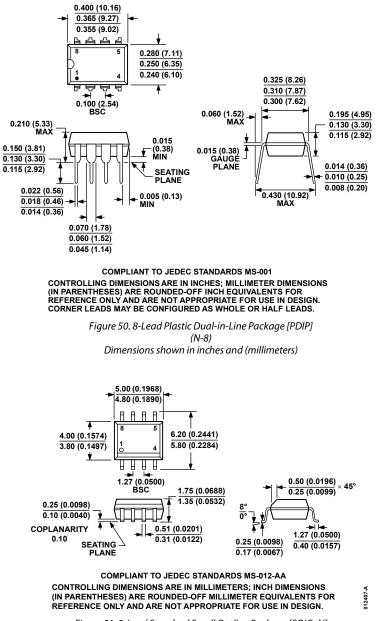
Figure 51. 8-Lead Standard Small Outline Package [SOIC\_N] (R-8) Dimensions shown in millimeters and (inches)
