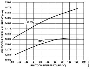
Figure 17. Supply Current vs. Junction Temperature
