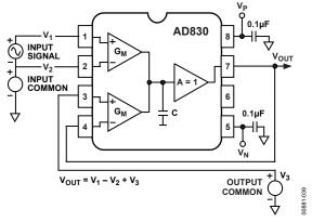
Figure 39. Differential Amplification with Level Shifting
