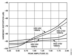
Figure 13. Harmonic Distortion vs. Peak Amplitude, Frequency = 100 kHz
