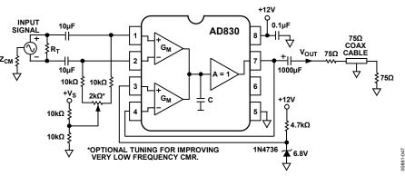
Figure 47. AC-Coupled Line Receiver
