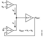
Figure 25. AD830 as a Difference Amplifier
