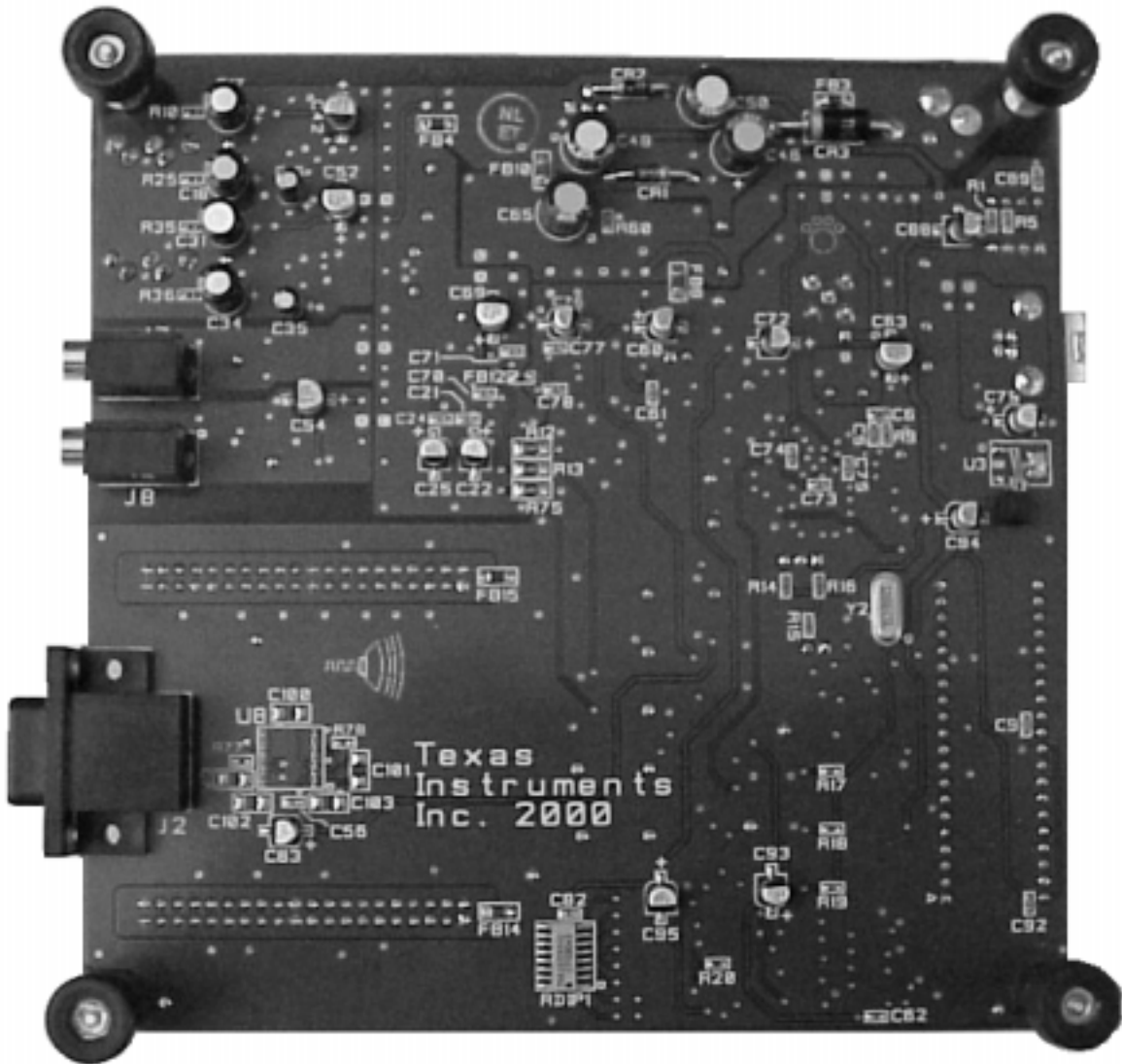
Figure 2–2. TAS1020A EVM Bottom View
