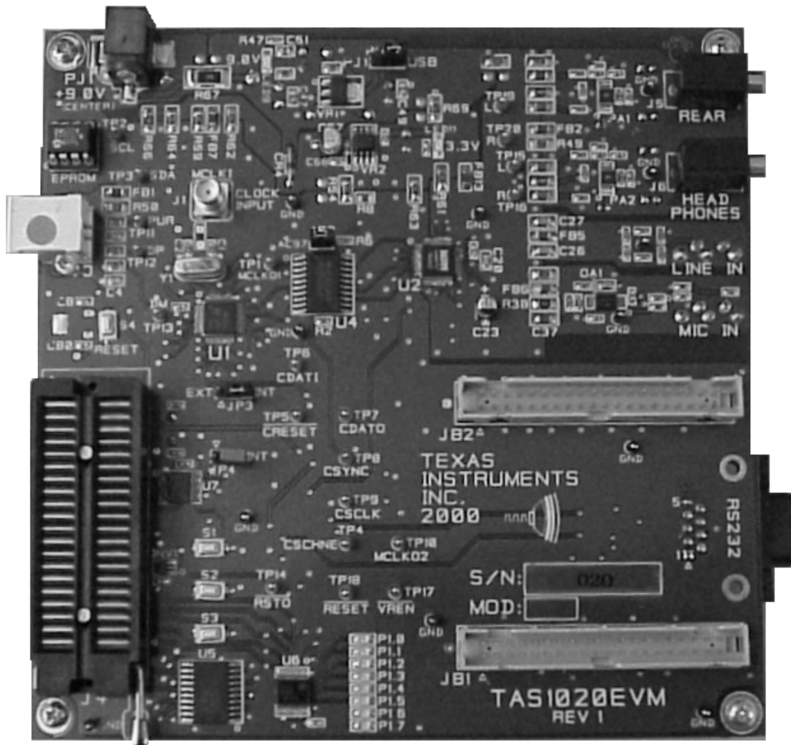
Figure 2–1. TAS1020A EVM Top View
