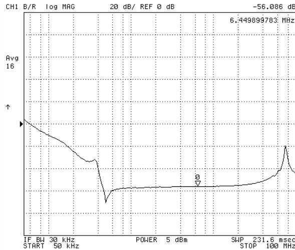
Figure 2 - Differential mode attenuation, 0.05-100 MHz. Source and load resistances are 50 \Omega . Vertical scale: 20 dB/div, with zero level marked by arrow. No load @ 25 ^{\circ} C
