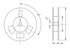
Devices are packed in accordance with EIA standard RS-481-A.
