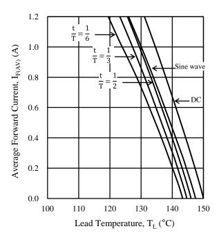
Figure 4. SARS01  $T_L$  vs.  $I_{F(AV)}$  Derating Curves  $(V_R = 800 \text{ V}, T_J = 150 \text{ °C})$
