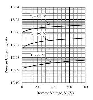
Figure 12. SARS05  $V_R$  vs.  $I_R$  Typical Characteristics
