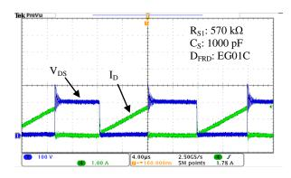
Figure 14. Waveforms of General Clamp Snubber Circuit
