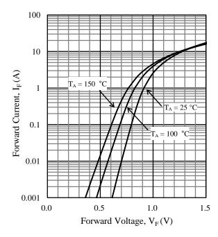
Figure 11. SARS05  $V_F$  vs.  $I_F$  Typical Characteristics
