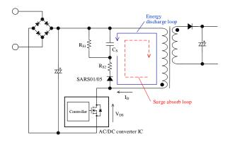
Figure 16. Clamp Snubber Circuit using SARS01/05
