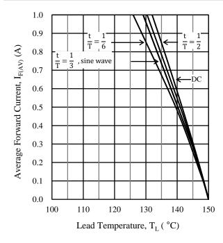
Figure 9. SARS05  $T_L$  vs.  $I_{F(AV)}$  Derating Curves  $(V_R = 0 \text{ V}, T_J = 150 \text{ °C})$
