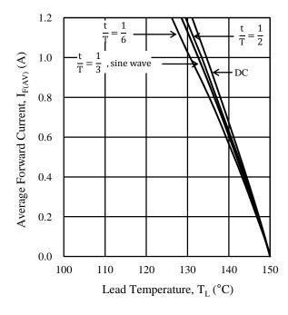
Figure 3. SARS01  $T_L$  vs.  $I_{F(AV)}$  Derating Curves  $(V_R = 0~V, T_J = 150~^{\circ}C)$
