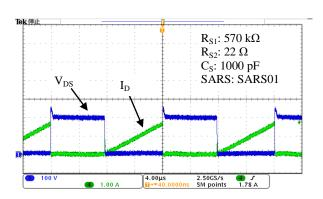
Figure 17. Waveforms of Clamp Snubber Circuit using SARS01
