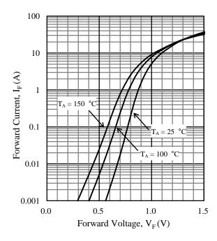
Figure 5. SARS01 V<sub>F</sub> vs. I<sub>F</sub> Typical Characteristics
