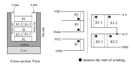
Figure 21. Winding Structure
