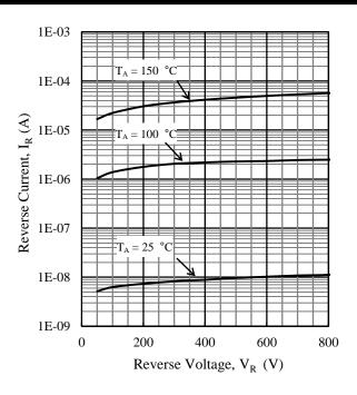
Figure 6. SARS01 V<sub>R</sub> vs. I<sub>R</sub> Typical Characteristics
