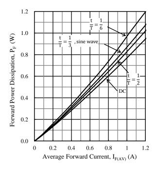
Figure 1. SARS01  $I_{F(AV)}$  vs.  $P_F$  Power Dissipation Curves  $(T_J = 150 \text{ °C})$
