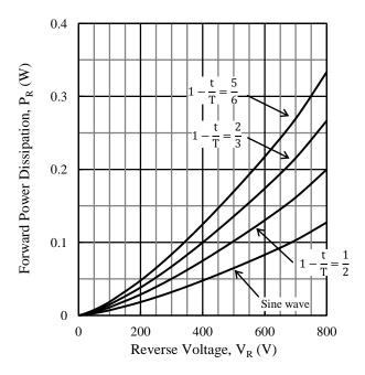
Figure 8. SARS05  $V_R$  vs.  $P_R$  Power Dissipation Curves  $(T_J = 150 \, {}^{\circ}\text{C})$
