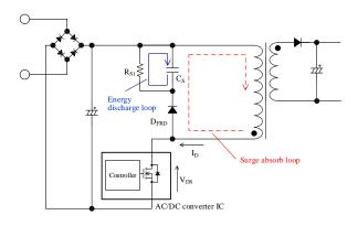
Figure 13. General Clamp Snubber Circuit
