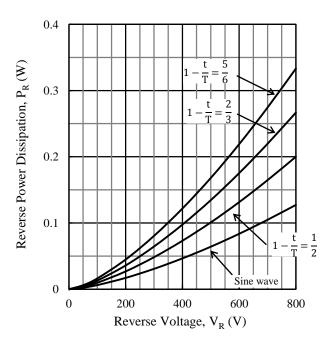
Figure 2. SARS01  $V_R$  vs.  $P_R$  Power Dissipation Curves  $(T_J = 150 \, {}^{\circ}\text{C})$
