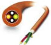
rugged PCF installation cable for inner areas with highly tear-proof aramid strain-relief elements. Individual elements made from highly flexible FRNC material. The cable is halogen-free, ozone and UV resistant and has a rugged polyurethane (PUR) outer sheath.
