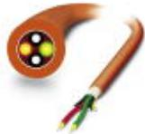
rugged PCF installation cable (IP20 heads only) for inner areas with highly tear-proof aramid strain-relief elements. Individual elements made from highly flexible FRNC material. The cable is halogen-free, ozone and UV resistant and has a rugged polyurethane (PUR) outer sheath.
