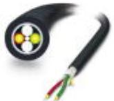
Highly rugged PCF round cable (IP20 heads only) for assembly and for outdoor installation with integrated moisture barrier as well as rodent-proof scrim. Individual elements made from highly flexible FRNC material. The wire is ozone and UV resistant with a very rugged polyethylene outer sheath.
