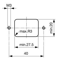
E: Solder terminals: 22.5 mm E: Quick connect terminals: 25.5 mm
