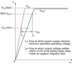
Figure 1: Definition of Power-On Time, t<sub>PO</sub>
