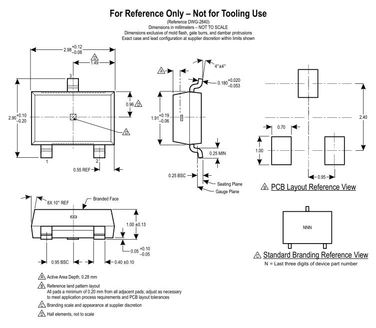
Figure 7: Package LH, 3-Pin (SOT-23W)
