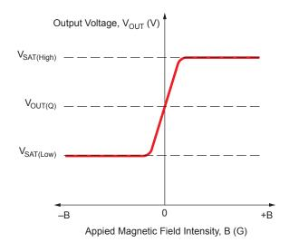
Figure 2: Effect of Saturation
