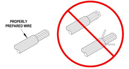
**Note**: Due to the delicate nature of this wire, care must be taken to gently touch the wire to the wire stop when crimping. The wire must be positioned directly above the terminal. Pushing the wire against the wire stop will result in strands out of the crimp. For semi-automatic crimping the operator may choose to lay the wire into the terminal for crimping.
