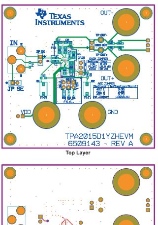
Bottom Layer Figure 2. TPA2015D1 EVM – Top and Bottom Layers
