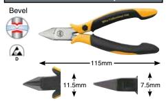
32706 Precision Cutters, Wide Tapered Head, Bevel Cutters drop-forged for an ideal material structure. Precise aligned cutting edges are additionally induction hardened at a hardness of Approx. 64°HRC. Two component non-slip soft grip handle, ESD Safe Dissipative. Item No. mm Inch Copper Head Wdth Ibs. Pkg. 115 4.5 32706 1.4 11.0mm .20 1
