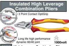
32820 High Leverage Combination Pliers. Insulation According to EN/IEC, ASTM, NFPA & CSA,  $\Leftrightarrow$  up to 1000 Volt. Extra long cutting edge for flat & round cables. Cutting edges additionally induction hardened to approx. 64HRC. C70 Special tool steel. Use for gripping, pulling & holding as well as cutting wires & cables ranging in hardness from soft to extremely hard.
