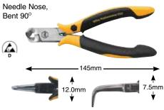
32748 ESD Safe Pliers, Needle Nose Pliers, Bent 90°, Smooth Jaws Pliers dropforged for an ideal material structure. Precisely aligned, jaws, hardened. Two component non-slip soft grip handle, ESD Safe Dissipative. mm Inch Head Wdth lbs. Pkg. 32748 145 5 3/4 12.0mm .21 1
