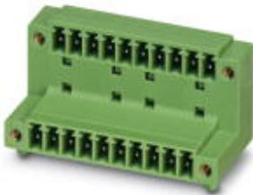
Header, Nominal current: 8 A, Rated voltage (III/2): 160 V, Number of positions: 2, Pitch: 3.81 mm, Color: green, Contact surface: Tin, Mounting: Wave soldering, In combination with MCV plug components, both an MCVW and an MCVR plug must be used.
