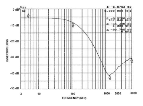
Figure 1. Insertion Loss vs. Frequency (FILTER1 Input to GND)
