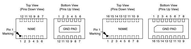
CM1409-06DE 12-Lead WDFN Package CM1409-08DE 16-Lead WDFN Package
