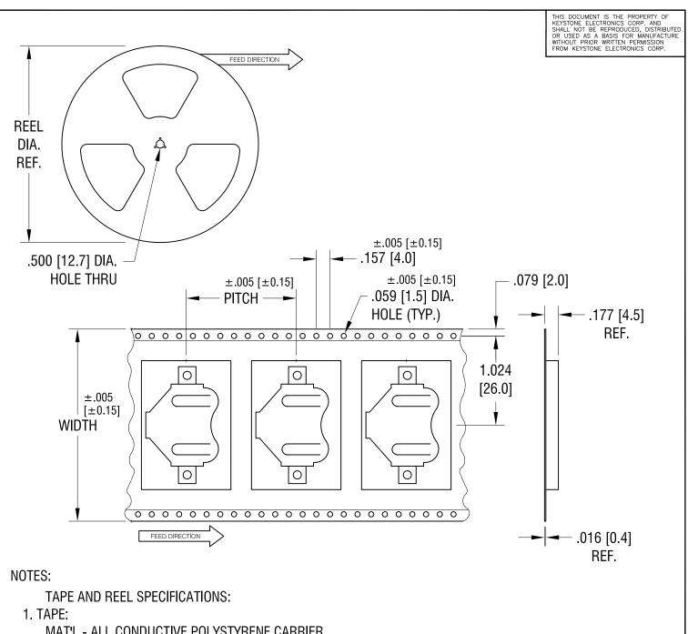
MAT'L - ALL CONDUCTIVE POLYSTYRENE CARRIER ANSI/EIA-481 STANDARD 2.205 [56.0] WIDE; 1.260 [32.0] PITCH
