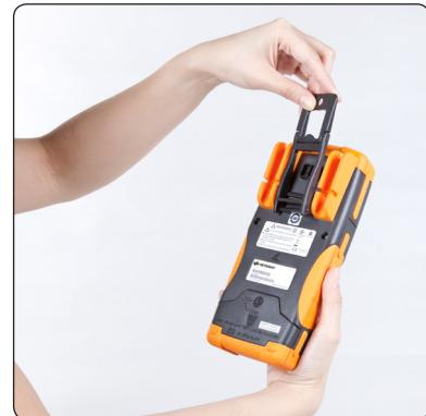
3) Press the stand down into its hinge.
