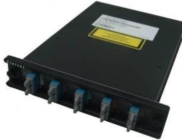
CWDM MUX/DEMUX-4-2 plug-in module is a passive optical multiplexer/demultiplexer designed to add and drop CWDM wavelength channels to an existing backbone ring. The module multiplexes and demultiplexes four CWDM wavelengths from a two-fiber ring, going in opposite directions into a network.
