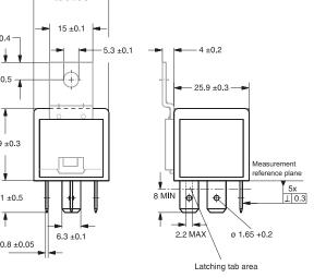
Quick connect terminal similar to ISO 8092-1 Power Relay F4 with PCB terminals
