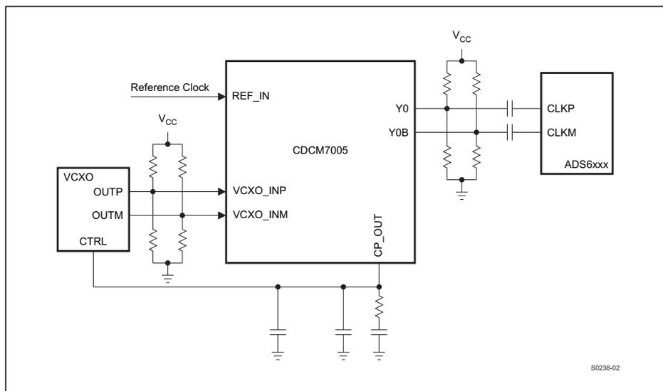
Figure 89. PECL Clock Drive Using CDCM7005
