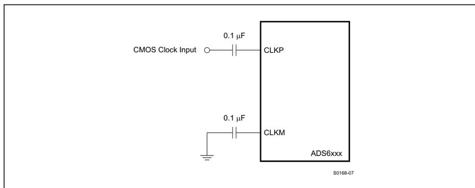
Figure 90. Single-Ended Clock Driving Circuit
