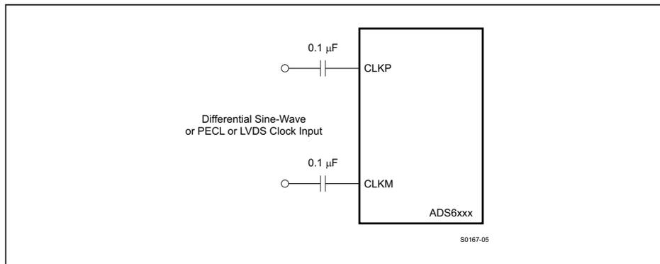
Figure 88. Differential Clock Driving Circuit
