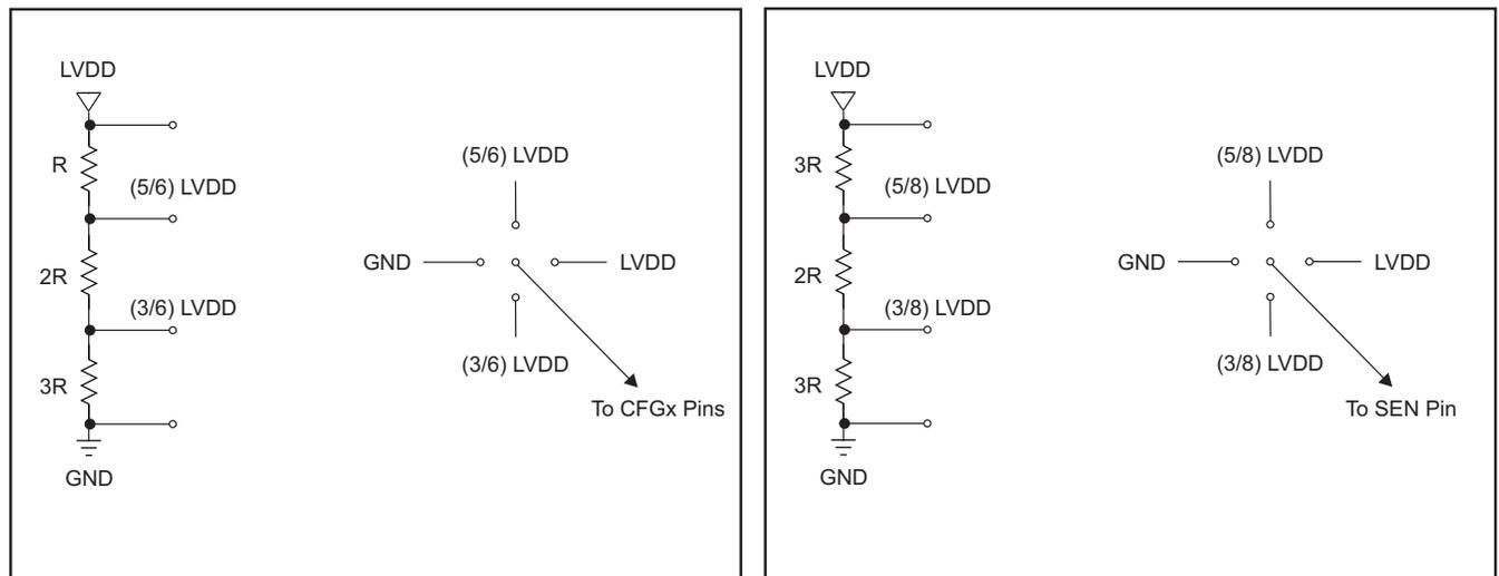
**Figure 3. Simple Scheme to Configure Parallel Pins**
