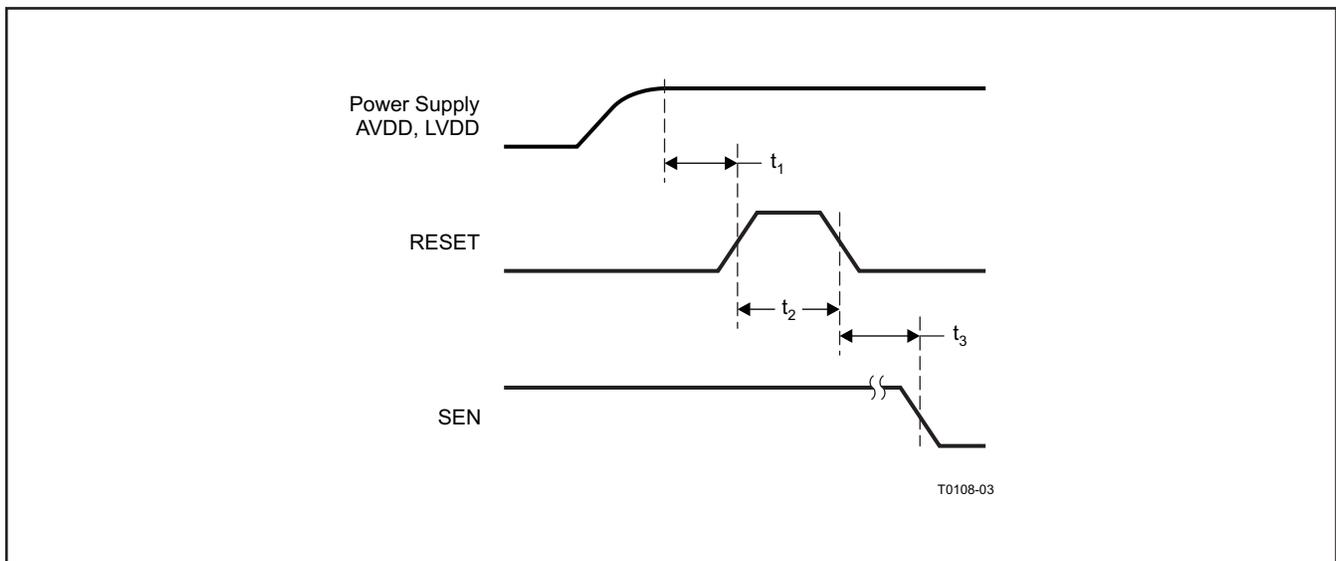
Figure 5. Reset Timing
