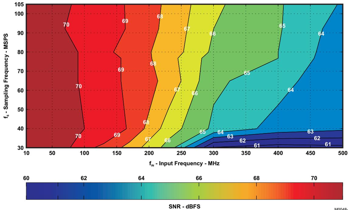
Figure 78. SNR Contour (3.5 dB coarse gain)
