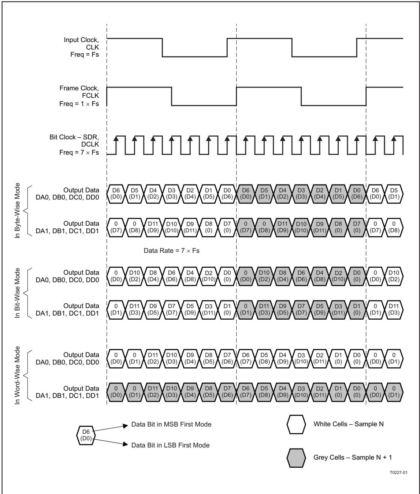
Figure 93. 2-Wire Interface 14x Serialization – SDR Bit Clock
