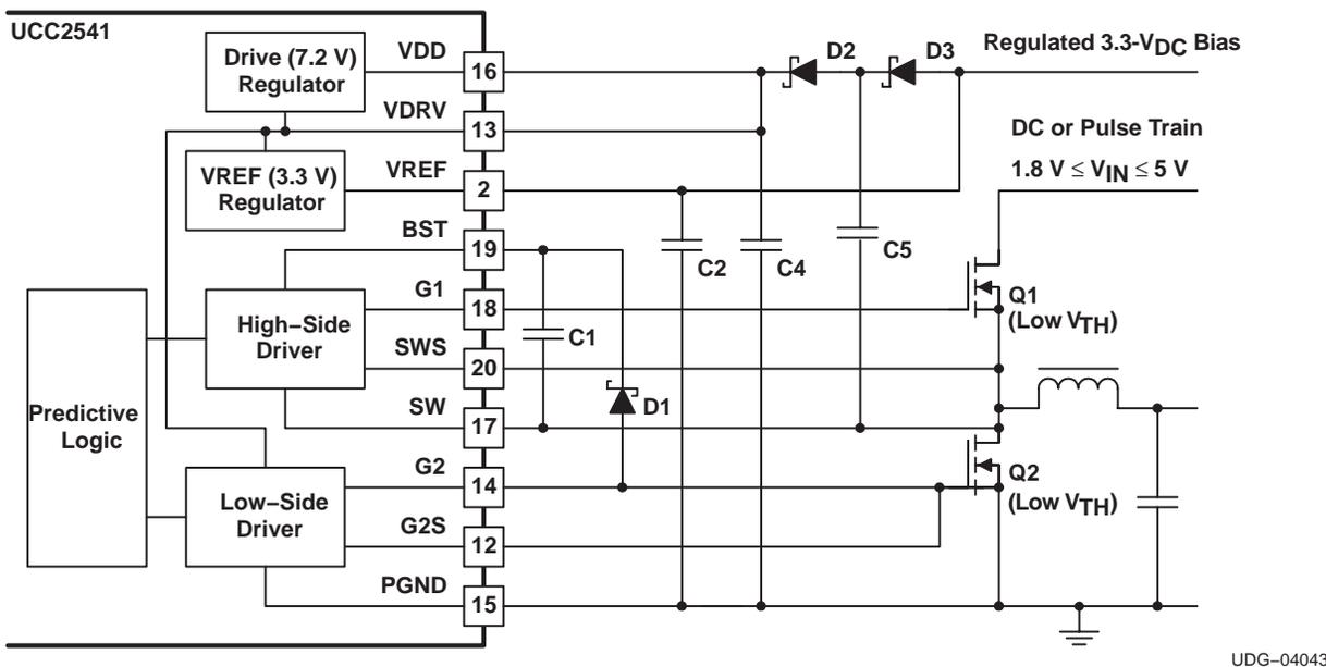
Figure 13. Mode 3 With Regulated 3.3-V<sub>DC</sub> Bias, Low Threshold Power MOSFETs
