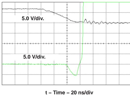
Figure 33. Predictive Gate Drive – G2 Falling
