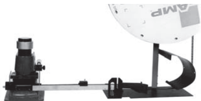
Manual Bench Tool with Applicator and Tape Feed Track
