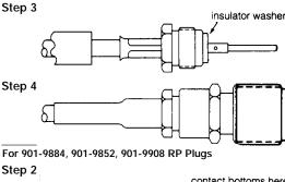
Step 3 Place insulator washer on cable center conductor and bottom against inner ferrule body as shown. Contact must butt firmly against insulator washer while soldering.
