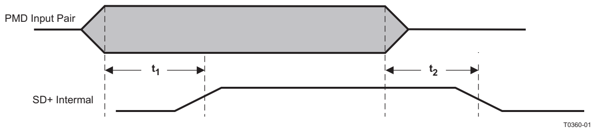
Figure 9-20. 100Base-TX Signal Detect Timing
