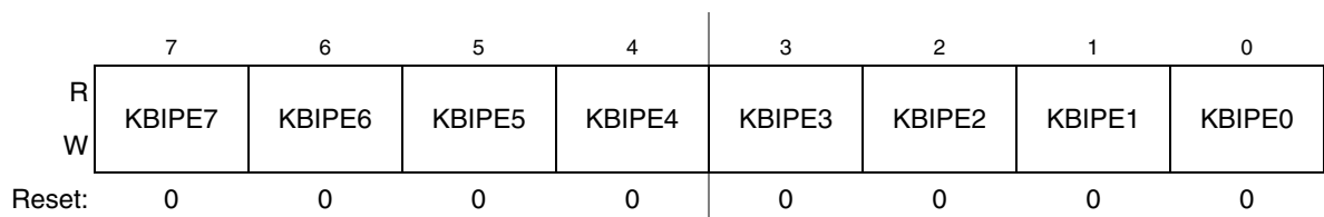
Figure 12-4. KBI Pin Enable Register
