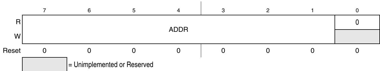
Figure 11-3. IIC Address Register (IICA)
