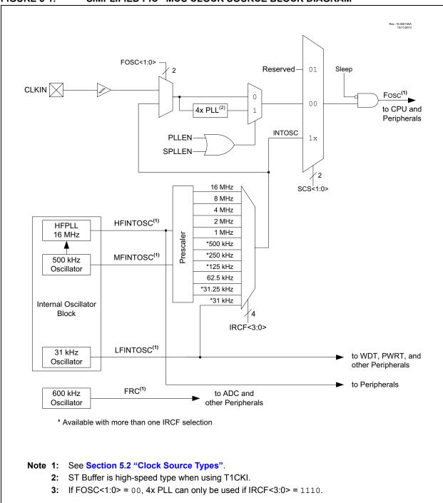
FIGURE 5-1: SIMPLIFIED PIC® MCU CLOCK SOURCE BLOCK DIAGRAM
