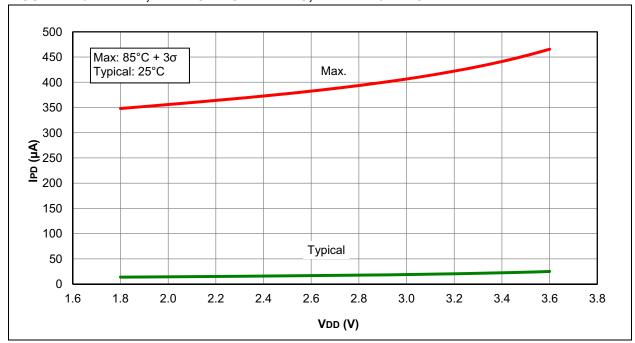
FIGURE 27-32: IPD, ADC NON-CONVERTING, PIC12F1571/2 ONLY
