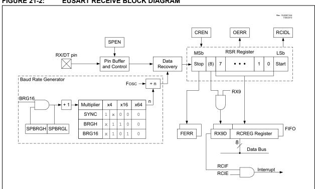
**FIGURE 21-2: EUSART RECEIVE BLOCK DIAGRAM**
