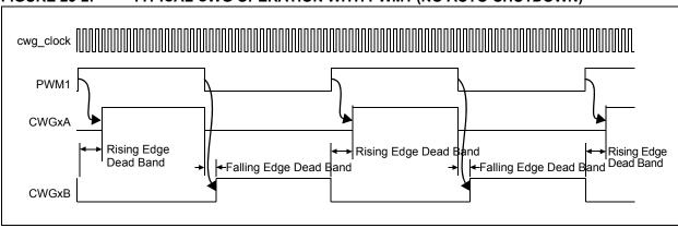
FIGURE 23-2: TYPICAL CWG OPERATION WITH PWM1 (NO AUTO-SHUTDOWN)
