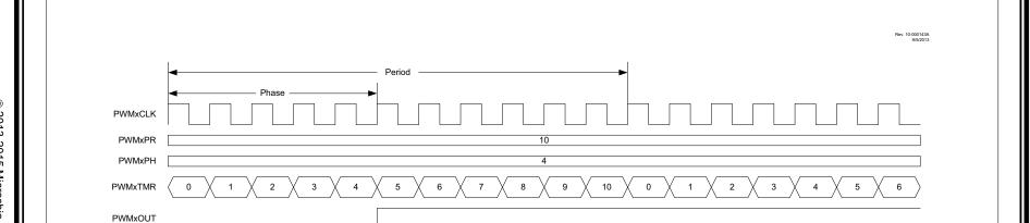
**SET ON MATCH PWM MODE TIMING DIAGRAM**
