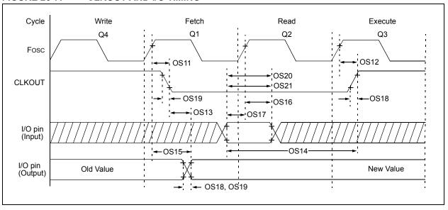
TABLE 26-10: CLKOUT AND I/O TIMING PARAMETERS
