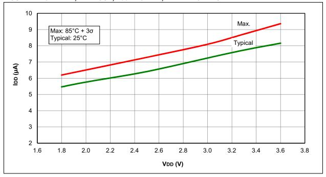
FIGURE 27-14: IDD, LFINTOSC, Fosc = 31 kHz, PIC12F1571/2 ONLY
