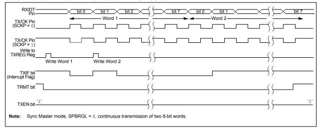
FIGURE 21-11: SYNCHRONOUS TRANSMISSION (THROUGH TXEN)
