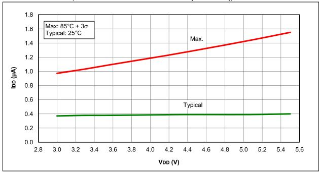
FIGURE 27-31: IPD, ADC NON-CONVERTING, PIC12LF1571/2 ONLY
