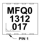
TABLE 29-1: 8-LEAD 3x3x0.9 DFN (MF) TOP MARKING
