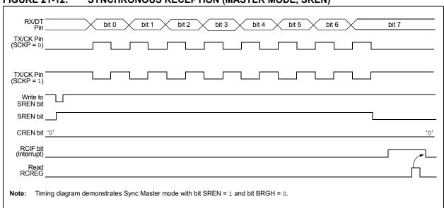
FIGURE 21-12: SYNCHRONOUS RECEPTION (MASTER MODE, SREN)
