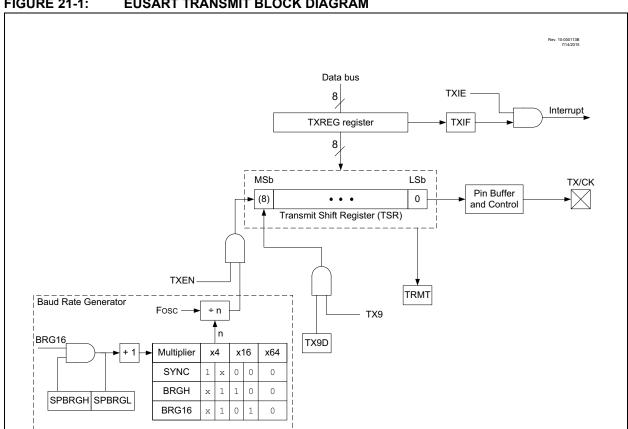
**FIGURE 21-1: EUSART TRANSMIT BLOCK DIAGRAM**
