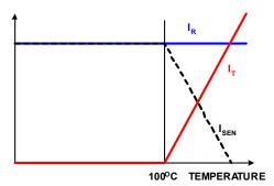
FIGURE 21. CURRENT SIGNALS AT THE AMPLIFIER CA INPUT
