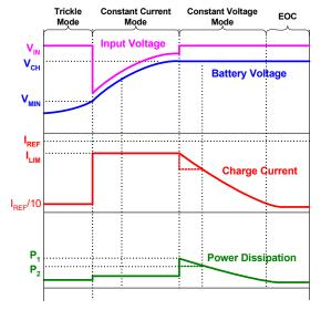
FIGURE 19. TYPICAL CHARGE CURVES USING A CURRENT-LIMITED ADAPTER
