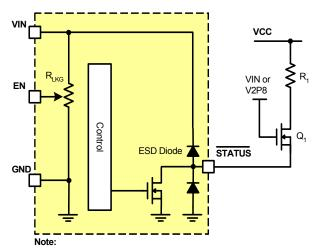
$R_{LKG}$  is approximately 240k $\!\Omega$  when EN is floating and is approximately 140k $\!\Omega$  when the EN is grounded.
