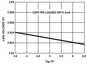
FIGURE 7. V2P8 OUTPUT vs INPUT VOLTAGE
