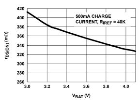
FIGURE 10.  $r_{\text{DS(ON)}}$  vs output voltage using current limited adapters
