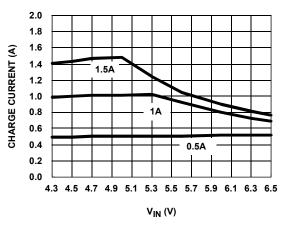
FIGURE 6. CHARGE CURRENT vs INPUT VOLTAGE
