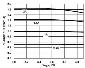
FIGURE 4. CHARGE CURRENT vs OUTPUT VOLTAGE
