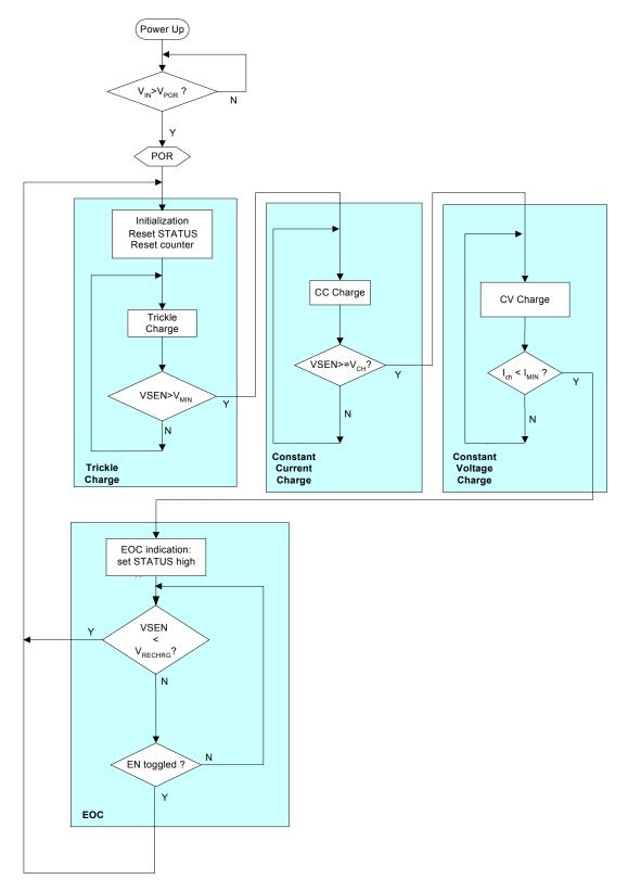
FIGURE 17. CHARGING STATE DIAGRAM
