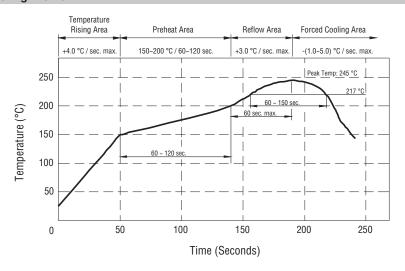
Peak Temperature: 245 °C max. Max. Peak Temperature: -5 °C, 30 sec. max. Max. Time Above 217 °C: 60 ~ 150 sec. max.
