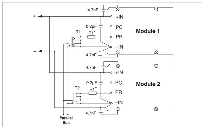
Figure 10 — Transformer-coupled interface
