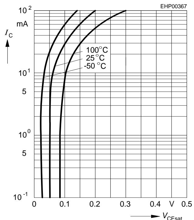
**Output characteristics  $I_C = f(V_{CE})$ ,**
