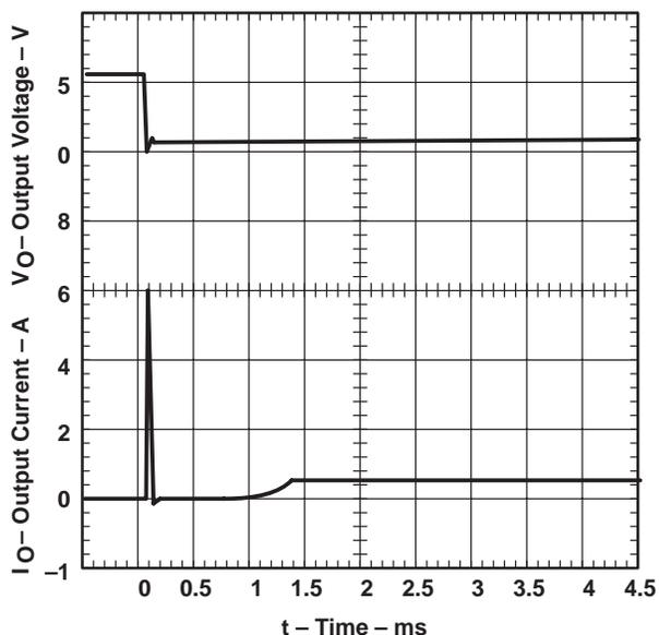
Figure 5. TPS2010, Short-Circuit Current.
