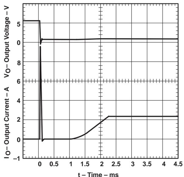
Figure 7. TPS2012, Short-Circuit Current.
