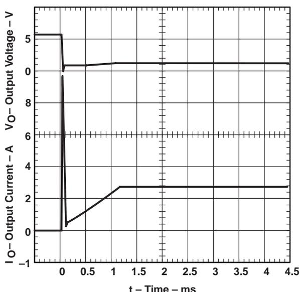
Figure 8. TPS2013 – Short-Circuit Current.
