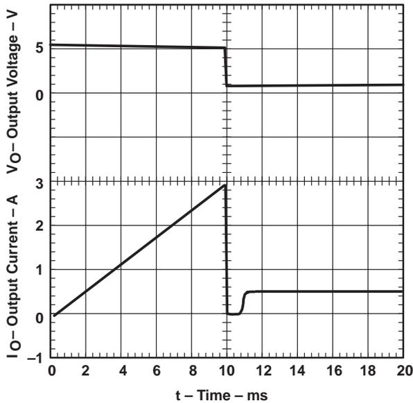
Figure 9. TPS2010 – Threshold Current,
