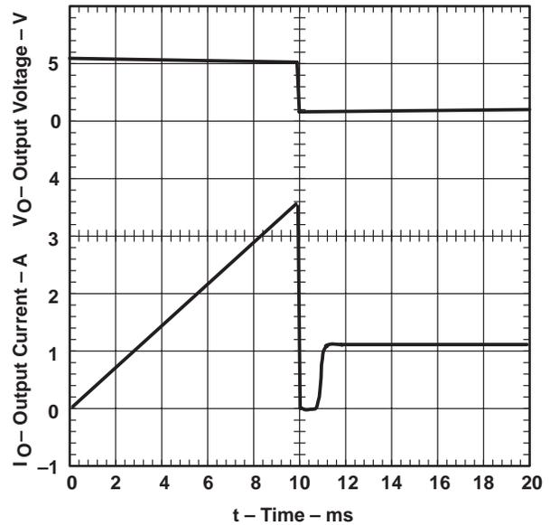
Figure 10. TPS2011 – Threshold Current,
