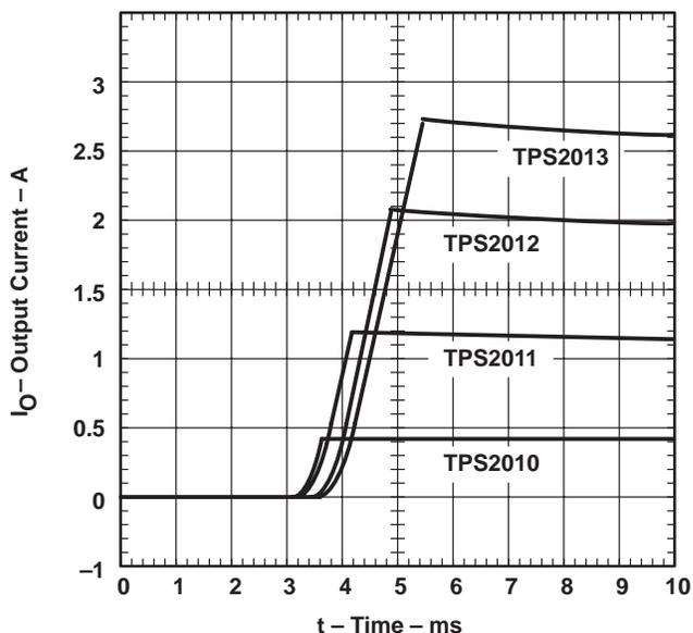
Figure 13. Turned-On (Enabled) Into Short Circuit,  $V_{I(IN)} = 5.5 V$
