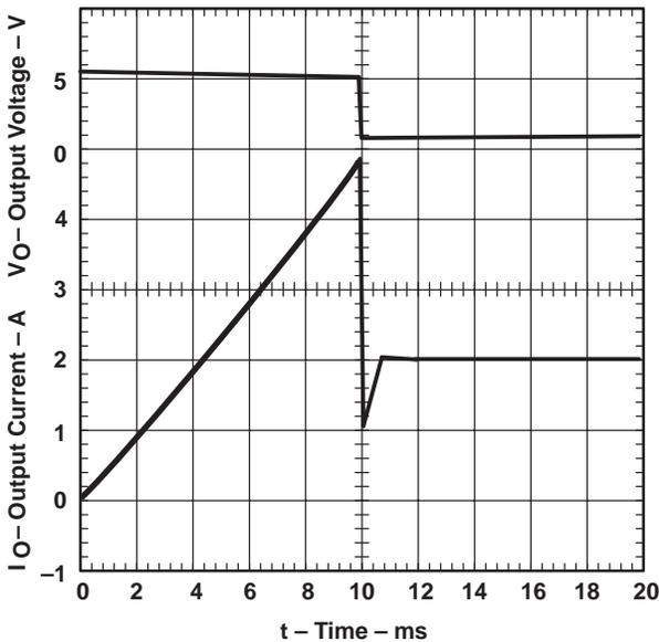
Figure 11. TPS2012 – Threshold Current,
