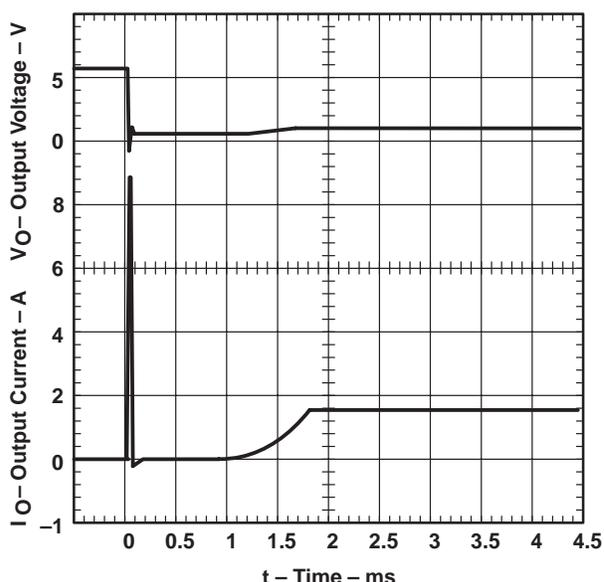
Figure 6. TPS2011, Short-Circuit Current.
