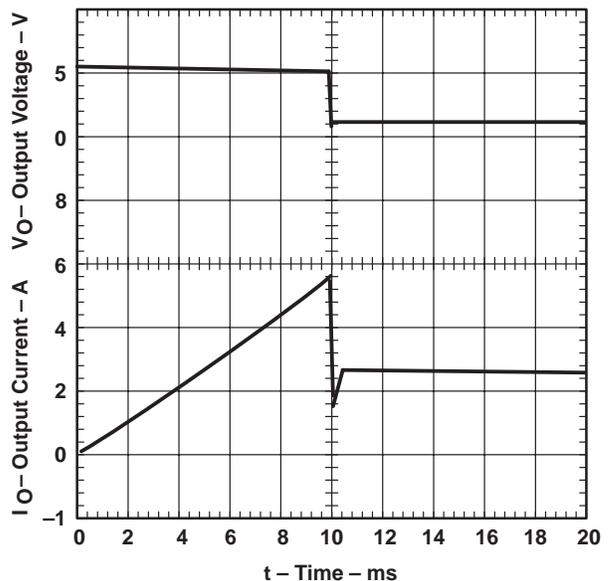
Figure 12. TPS2013 – Threshold Current,
