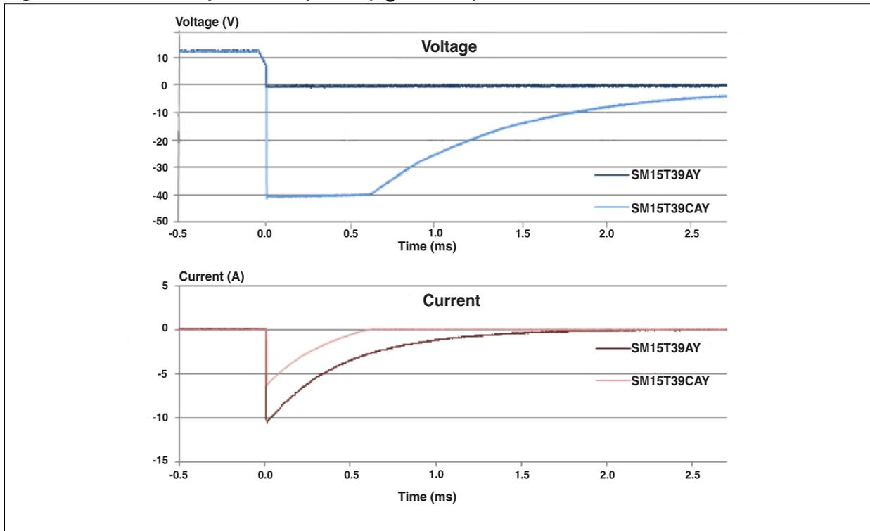
Figure 13. ISO7637-2 pulse 2 response ( $V_S = 50\text{ V}$ )
