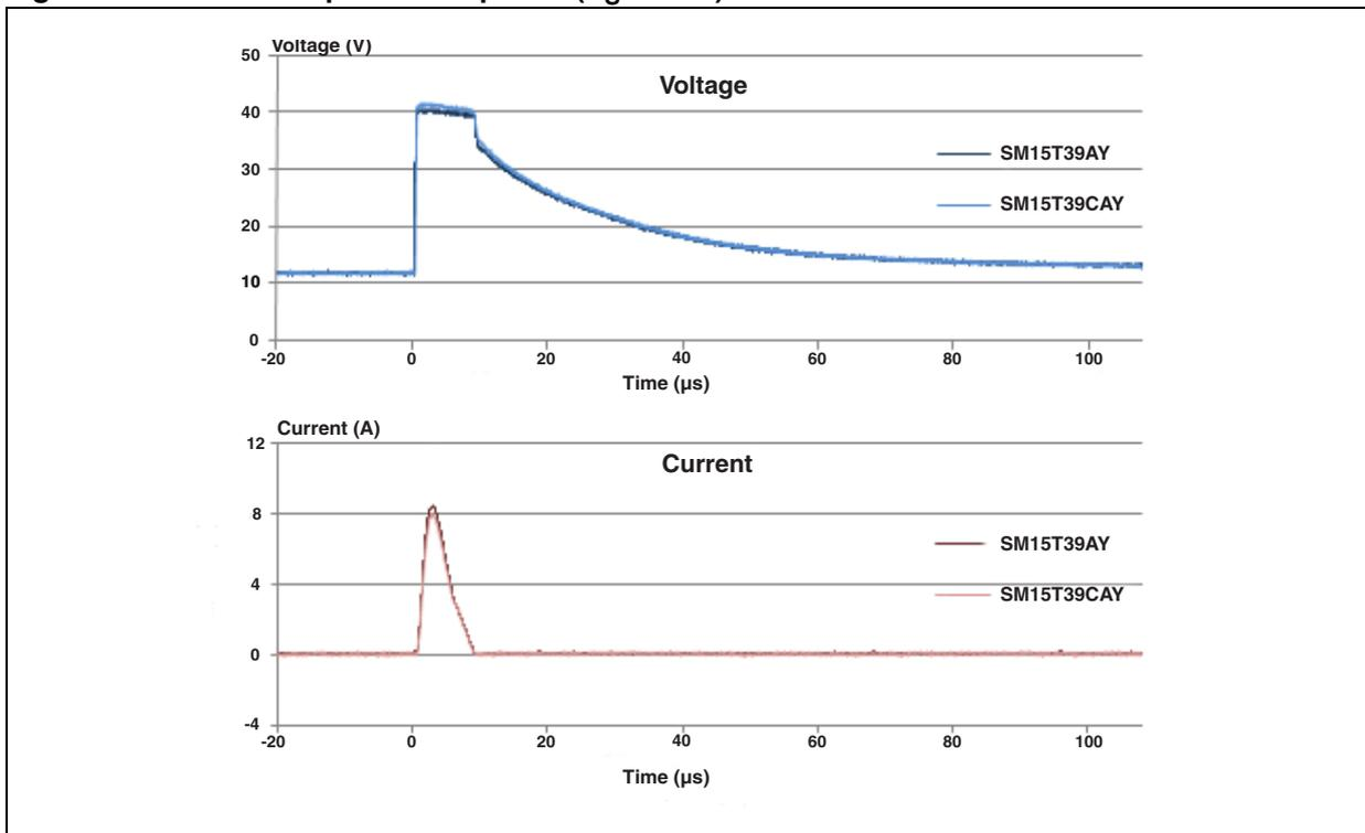
Figure 14. ISO7637-2 pulse 3a response ( $V_S = -150\text{ V}$ )
