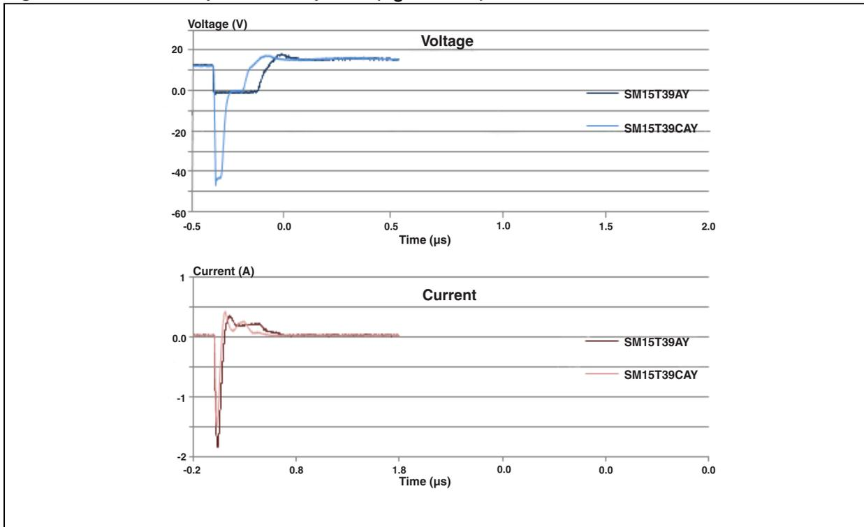
Figure 15. ISO7637-2 pulse 3b response ( $V_S = 100\text{ V}$ )
