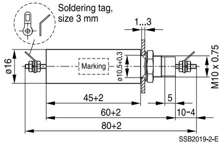
Tightening torque: 3 +0.5 Nm
