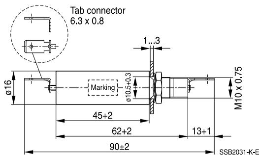
Tightening torque: 3 +0.5 Nm
