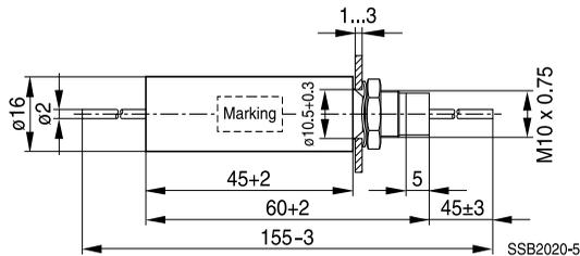
Tightening torque: 3 +0.5 Nm
