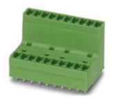
Header, Nominal current: 8 A, Rated voltage (III/2): 160 V, Number of positions: 14, Pitch: 3.81 mm, Color: green, Contact surface: Tin, Mounting: Wave soldering, In combination with MCV plug components, both an MCVW and an MCVR plug must be used.
