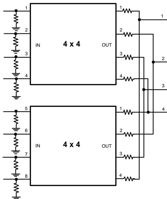
**Figure 45. Input Expansion with Separate Termination Resistors**
