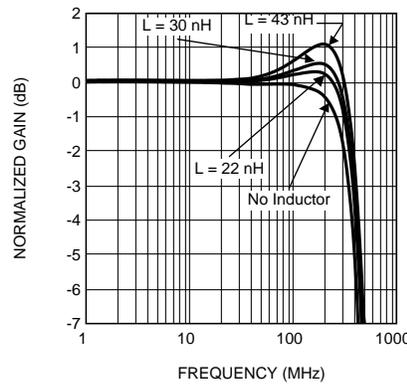
Figure 48. Termination Inductor Bandwidth Enhancement Using Input 0
