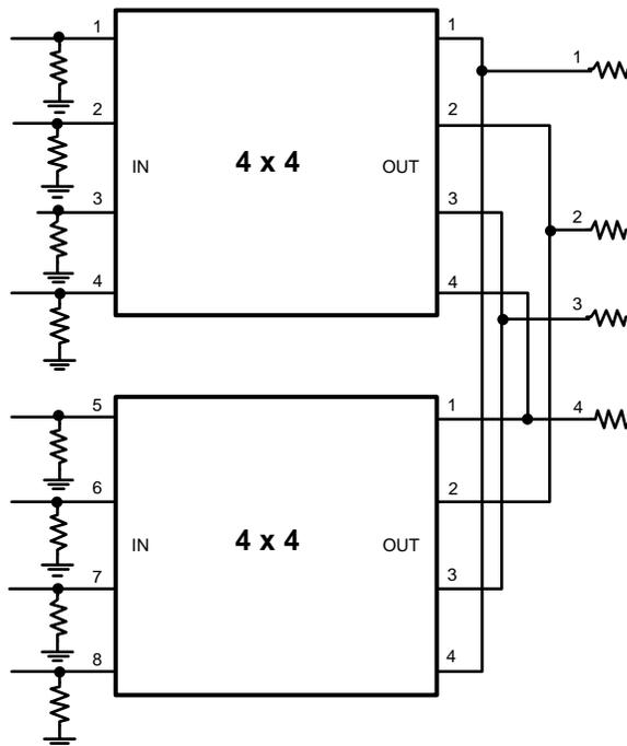
**Figure 44. Input Expansion with Shared Termination Resistors**
