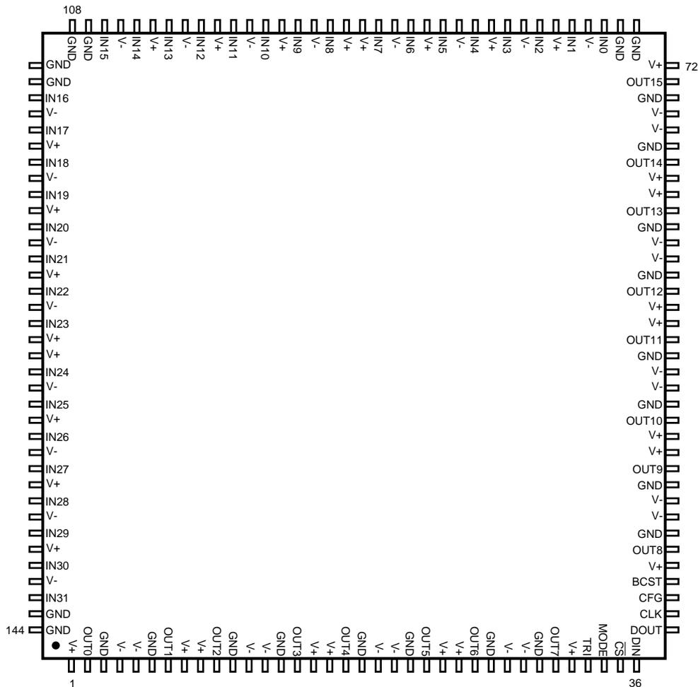
Figure 1. 144-Pin LQFP Package
