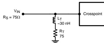
Figure 47. Use of Termination Inductor to Increase Bandwidth
