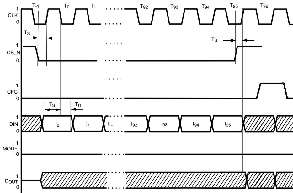
Figure 54. Timing Diagram for Serial Mode
