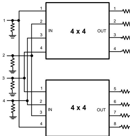
Figure 43. Output Expansion no Buffers
