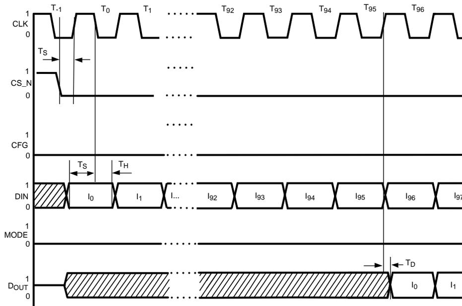
Figure 56. Timing Diagram for Daisy Chain Operation
