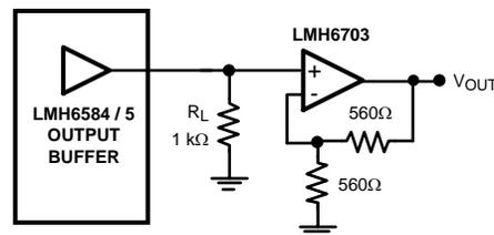
**Figure 52. Buffered Output**
