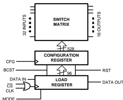
**Figure 53. Block Diagram**
